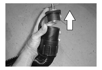
3. Place the FaST PAK carton in the carton holder located next to the seat. Connect the supply hose to the FaST PAK bag.
