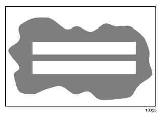
If one, or both of the brush patterns are tapered, the brushes need adjustment to straighten the brush pattern.
