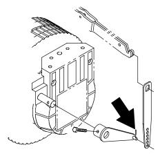
Insert the cotter key back into the brake extension arm, and check the brake for proper operation.
