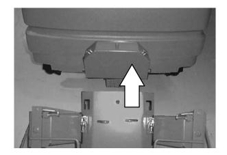
4. Fasten the latches on the front of the mountng bracket. Release the parking brake and drive to the designated area to be swept.
