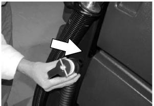
13. Check the vacuum fan inlet filter daily. Clean inlet filter with a damp cloth or hose when dirty. Allow filter to dry completely before replacing it into machine.
