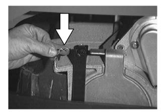
16. Cylindrical scrub head: Remove and clean the debris trough. Place the trough back in the scrub head when clean.
