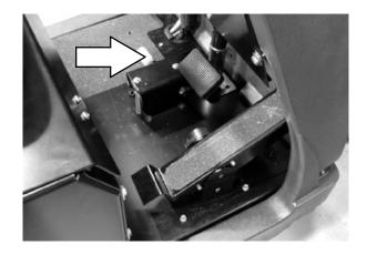
3. Lower the scrub head in the chalked area. Allow the machine to scrub in the same place for 15 to 20 seconds.
