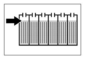
Using a hydrometer, measure the specific gravity to determine the charge level and condition of the batteries. If one or more of the battery cells test lower than the other battery cells (0.050 or more), the cell is damaged, shorted, or is near failure. Completely recharge the batteries, then retest them.
