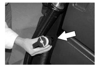
10. ES mode (option): Remove the drain hose cap while holding the hose up, then slowly lower the drain hose to the floor drain.
