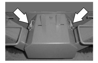
5. Pull the release lever to raise or lower each side of the *QuickMop*.
