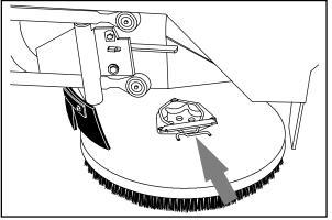
*Heavy duty stripping pad* – This black pad is for stripping floors. Cuts through old heavy finishes easier, to prepare the floor for re-coating.
