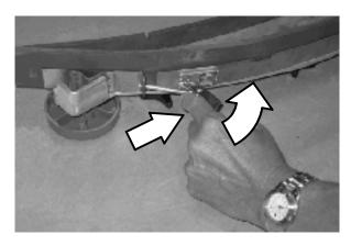
13. Reinstall the rear squeegee under the squeegee mount bracket and tighten all four knobs.
