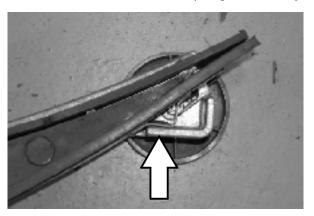
12. Tighten the rear squeegee retaining band tension latch.
