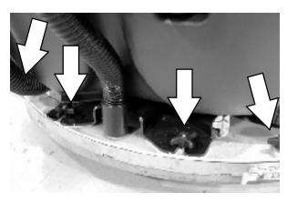
14. Reinstall the squeegee suction hose onto the rear squeegee assembly.
