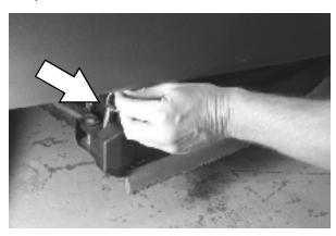
4. Open the side squeegee retainer pivot toward the front of the machine, then pull the side squeegee toward the rear of the machine to access the scrub brushes or pads.
