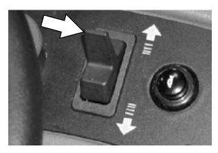
NOTE: The squeegee automatically raises when the machine is driven backwards. This prevents damaging the squeegee. When the machine is placed in reverse, the vacuum fan will shut off after a short delay.
