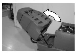
12. Flush the solution tank and rinse the float sensor located inside the back part of the solution tank. Rinse the screen filter on the bottom of the tank.
