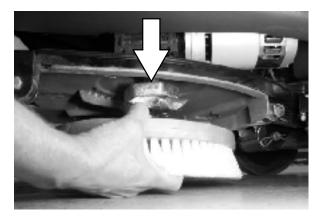
6. Place the new scrub brush/pad driver onto the drive hub. Ensure that it is securely mounted onto the brush drive hub.
