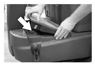
16. Replace the solution tank drain hose cap and mount the drain hose back onto the mounting clip after after the tank is drained.
