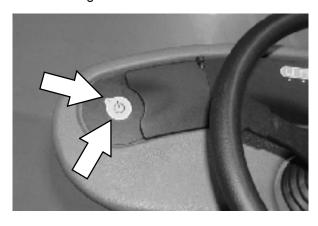
NOTE: Open the control panel cover to adjust the Brush Pressure and Solution Flow Setting while scrubbing if necessary.
