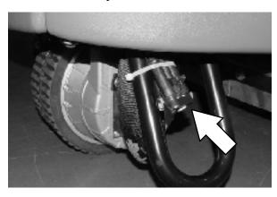
To disengage the brake, insert the tip of a small screw driver between the electronic brake lever and the hub.
