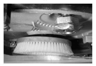
**Non-scuff polypropylene scrub brush** – This brush uses a softer, general purpose polypropylene bristle to lift lightly compacted soilage without scuffing high-gloss coated floors.
