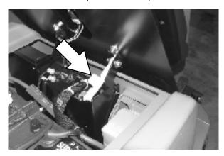
4. Remove the recovery tank drain hose. While holding the hose up, remove the plug, then slowly lower the drain hose to the floor drain or sink.
