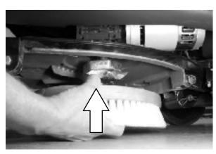
7. Close the side squeegee and the retainer pivot, then insert the pin.
