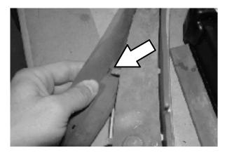
11. Reinstall the rear squeegee retaining band onto the squeegee assembly. Be sure each of the flanges on the retaining band are seated in the cut outs in the rear squeegee assembly.
