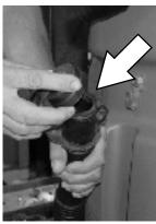
Tilt the recovery tank back to access the solution tank. Make sure the recovery tank is empty before tilting.
