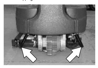
NOTE: It may be necessary to install tie-down brackets to the floor of the trailer or truck.
