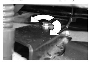
Turn the squeegee leveling bolt counter-clockwise to increase the deflection at the ends of the squeegee.
