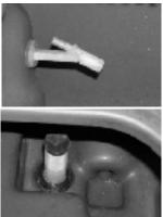
13. Carefully push the recovery tank forward to close the solution tank.
