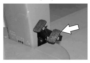
Release the propel pedal to stop the machine. Scrubbing functions stop and the automatic park brake will engage when the machine stops.
