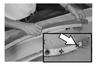
Install the new front squeegee blade or rotate the existing blade to the new edge. Be sure the holes in the front squeegee blade are hooked onto the tabs on the front blade clamp.
