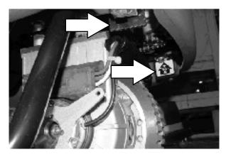
Rear jacking locations are located on both sides of the machine at the axles.
