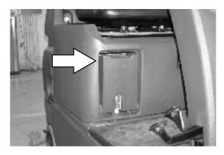
4. Squeeze the button on the FaST supply hose connector, then pull the empty FaST-PAK out from the compartment.
