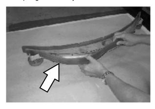
Loosen the two outer knobs on the rear squeegee assembly. Remove the front squeegee blade from the squeegee assembly.
