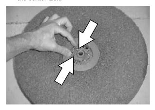
3. Flip or replace the scrub pad, center the scrub pad on the pad driver. Then reinstall the center disk to secure the pad in place on the pad driver.
