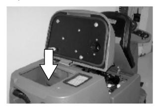
6. Rinse the float sensor located inside the recovery tank.
