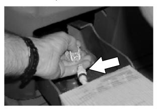
Remove the perforated knock outs from the new FaST-PAK carton. Do Not remove the bag from the carton. Pull out the hose connector located on the bottom of the bag and remove the hose cap from the connector.
