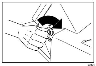
2. Raise the hopper slightly to release the hopper support bar.
