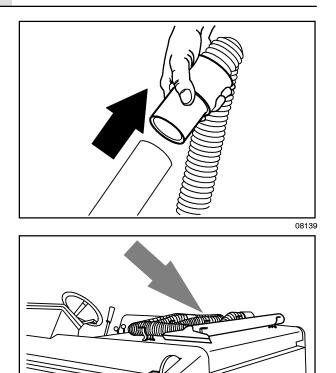
25. Put the vacuum wand and hose in the mounting clips.
