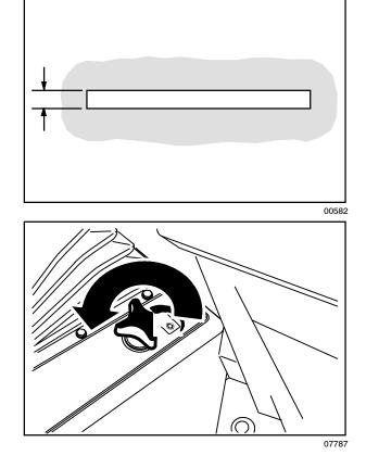
To decrease the width of the main brush pattern, turn the main brush down pressure knob clockwise.
