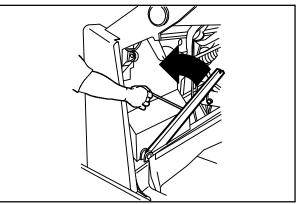
5. Slowly lower the hopper so the lift arm rests on the support bar.
