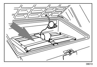
3. Disconnect the shaker motor wire connectors.
