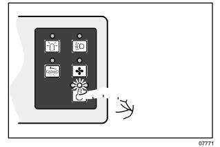
Fast 2: Press the engine speed switch until the third indicator light comes on. This speed is for sweeping light litter.
