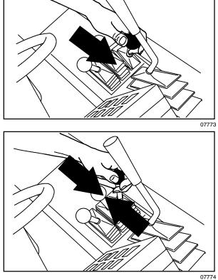
Main Brush On: Pull the main brush and side brush lever into the **On** position.
