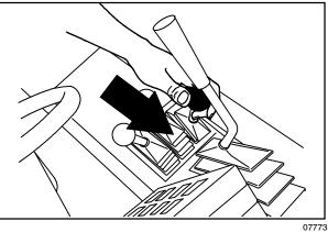
14. Press the vacuum fan switch to start the vacuum.
