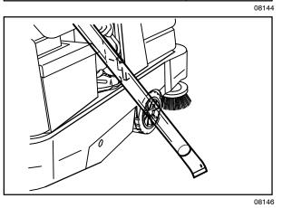
The operator can rest the wand on the side bracket.
