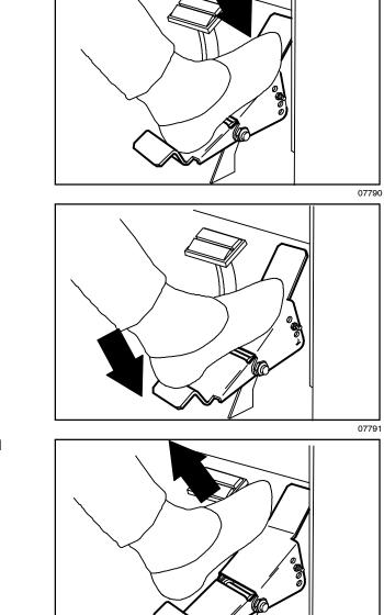
Reverse: Press the bottom of the directional pedal with the heel of your foot.
