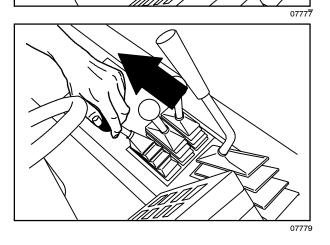
5. Release the hopper lift lever up and into the middle (Hold) position.
