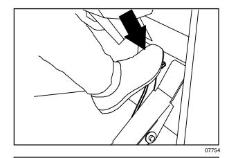
3. Select the (Idle) position with the engine speed switch.
