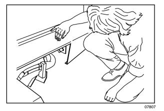
Check the engine air filter indicator.
