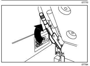
Turn the ignition switch key counter-clockwise to stop the engine. Remove the switch key.
