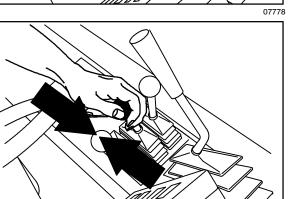
4. Pull the hopper lift lever into the **Up** position and raise the hopper to the desired height.
