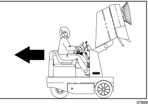
11. Push the hopper lift lever into the **Down** position.
