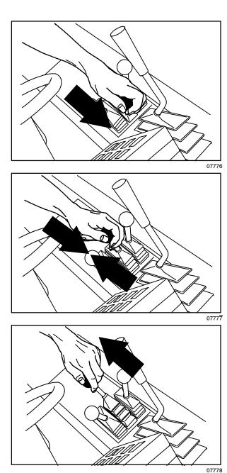
Close: Pull and hold the hopper door lever into the **Close** position.
