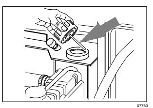
Check the engine oil level.
