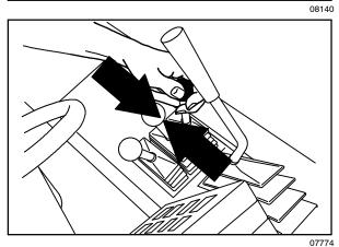
17. Press the vacuum switch to shut off the vacuum.
