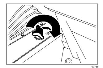
If the main brush pattern is tapered, more than 15 mm (0.5 in) on one end than the other, adjust the taper with the taper adjustment bracket at the drive end of the brush.
