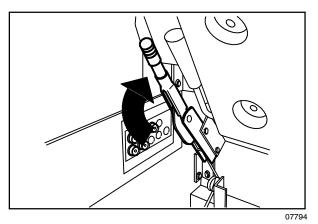
Release: Push the parking brake lever down.
