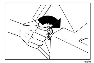
11. Select the (Fast 2) engine speed with the engine speed switch.
