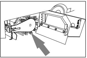
**Nylon 24-row Main Brush** – Recommended for severe dust conditions on rough surfaces. This brush has excellent pickup and long life.
