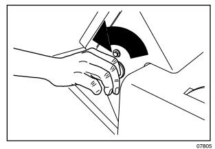
3. Turn the ignition switch key clockwise until the engine starts.
