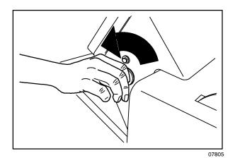
Start: Turn the key all the way clockwise. Release the key as soon as the engine starts.
