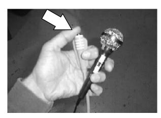
Press the top of the voice box switch to play the recorded message back continuously.
