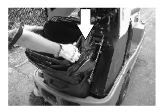
16.Check that the hopper track guides are resting properly on the hopper tracks on both sides of the debris hopper.
