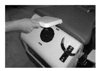
4. Lift the steering assembly off the front notched steering plate. Unfold the steering assembly back over the machine seat.
