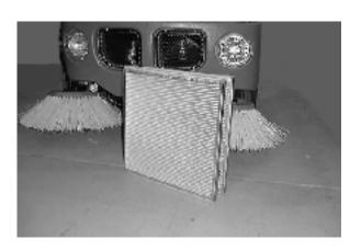
7. Clean the diffuser screens in the bottom of the filter housings and check for damage.
