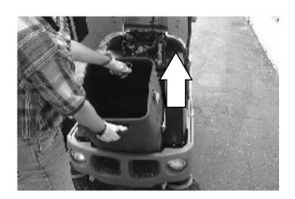
13.Clean the inside of the hopper compartment by scraping any compacted debris with a scraper. Use a stiff broom or brush to clean the vacuum screen.
