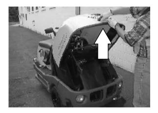
3. Pull on the cover prop rod to lock cover in open position.
