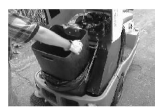
9. Unplug hopper drain plug to remove any excess water from the hopper.
