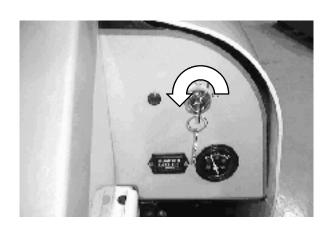
6. Turn the ignition key clockwise until the engine starts.
