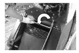
8. Pull hopper down towards front of machine and remove bag liner.
