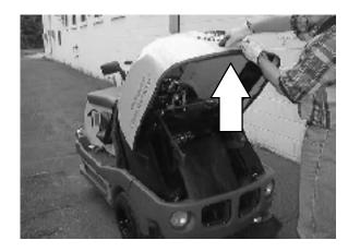
6. Pull on the cover prop rod to lock cover in open position.
