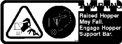
HOPPER SUPPORT BAR LABEL - LOCATED ON THE HOPPER SUPPORT BAR AND ON BOTH HOPPER LIFT ARMS.
