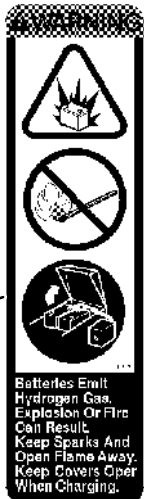
BATTERY CHARGING LABEL - LOCATED ON THE RELAY PANEL NEXT TO THE BATTERIES.
