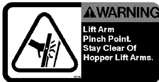
HOPPER LIFT ARM LABEL - LOCATED ON THE HOPPER COVER.
