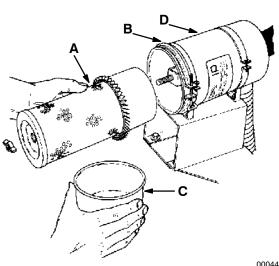
REMOVING AIR FILTER ELEMENT
