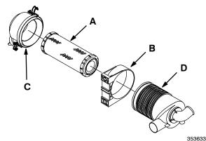
REMOVING AIR FILTER ELEMENT
