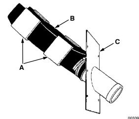
CORRECT POSITIONING OF LOWER SPRAY DEFLECTOR
