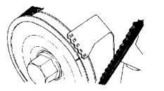
CRANKSHAFT PULLEY TIMING MARK
