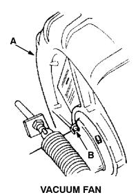
A. Vacuum Fan B. Grease Fitting 03789
