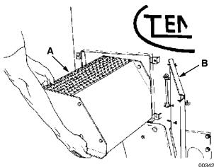
**REMOVING LAMINAR TUBES**
