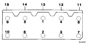
CYLINDER HEAD BOLT TIGHTENING SEQUENCE - CONTINENTAL ENGINES (For machines below serial number 006409)
