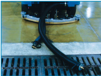
Use the drop down drain hose to empty the solution recovery tank into floor drain or sink.
