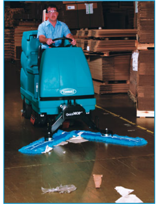
The optional QuickMop™ feature attaches to the front of the scrubber and allows the operator to sweep prior to scrubbing, which increases cleaning productivity.
