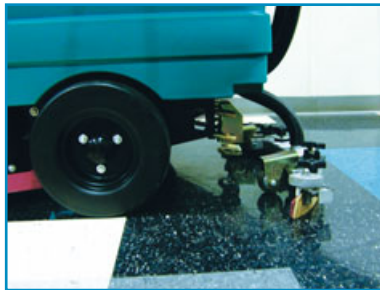
Breakaway squeegee prevents damage to walls and squeegee.
