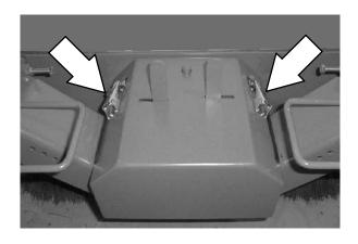
5. Pull the release lever to raise or lower each side of the *QuickMop*.
