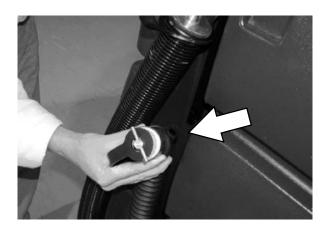
10. ES mode (option): Remove the drain hose cap while holding the hose up, then slowly lower the drain hose to the floor drain.
