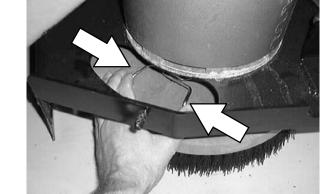
14. Check to make sure the brush is securely mounted on the brush drive hub.
