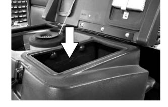
9. ES mode (option): Lift the solution tank draining hose off the lower retaining hook.
