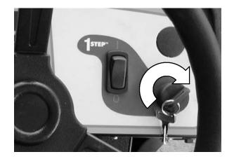
3. Turn the machine power off. See the STOP THE MACHINE section of the manual.
