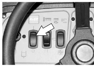
6. Press the top of the *one step switch* to start the scrubbing operations. See the ONE STEP SWITCH section of the manual.
