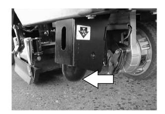
Jack up the rear of the machine from underneath the rear corners. Use a piece of wood between the jack and the frame to distribute the machine weight load.
