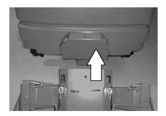
Fasten the latches on the front of the mounting bracket. Release the parking brake and drive to the designated area to be swept.
