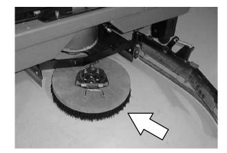
12. Line up the brush /pad driver socket with the drive plug.
