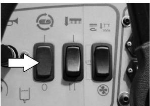
5. FaST SCRUBBING (option): Press the FaST switch to enable the FaST system. See the FaST SWITCH section of the manual.
