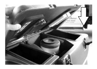
15. Cylindrical scrub head: Lower the scrub head approximately 25mm (1 in). Remove the cotter pin that holds the side squeegee in place on the right hand side of the machine. Swing the squeegee away from the scrub head.
