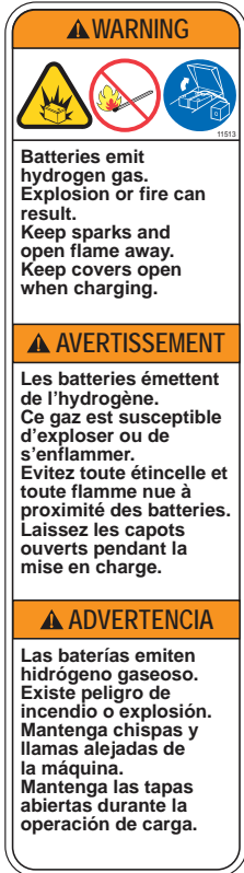
Located on front electrical access panel.
