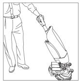
Lift up the scrub deck slowly until it's standing upright on the front wheels; guide the body towards the scrub deck until it snaps into a resting position.
