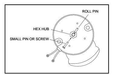
**6.** Release brush from spring tension. Remove screw connecting brush wire lead to brush holder. Clean brush holder to insure free movement.
