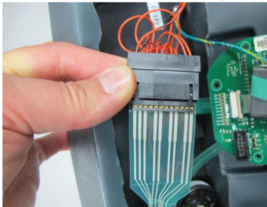
8. Release the control panel ribbon connection and pull the ribbon free. Gently pull ribbon out of the ferrite bead.
