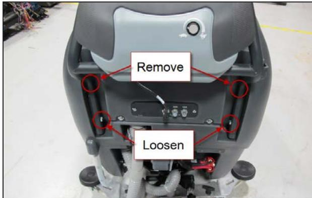
4. Disconnect handle wiring lead (Note photo is of early build).
