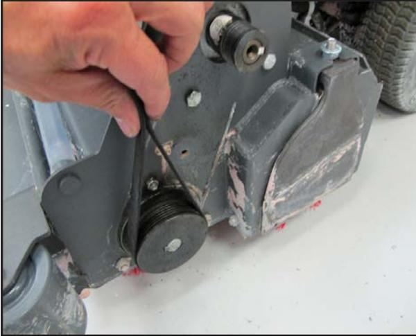
4. Use a screwdriver to pry the belt onto the motor pulley using a rolling action.
