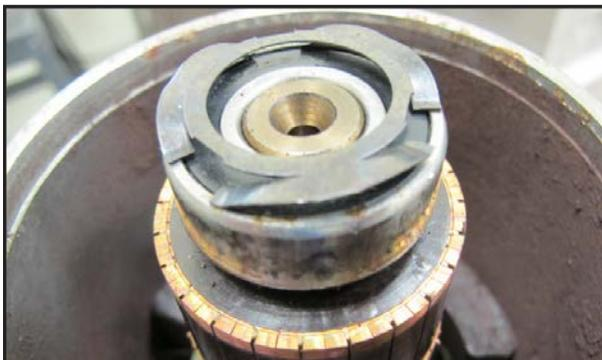
7. Install the end cover in stages, aligning the marks made earlier.
