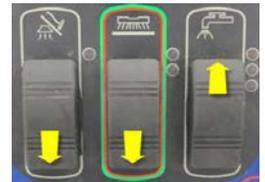
The Heavy Scrub Pressure Indicator will remain on and the Fault Indicator will be flashing a numeric value that represents the current setting. To change the setting, press the solution switch forward to increase the value or backwards to decrease the value. To save the setting, press the scrub switch forward (All LEDs will turn on) then turn off the key switch.
