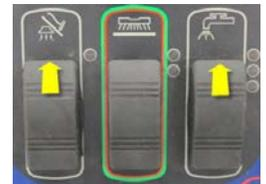
The Medium Solution Flow Indicator will remain on and the Fault Indicator will be flashing a numeric value that represents the current setting. To change the setting, press the solution switch forward to increase the value or backwards to decrease the value. To save the setting, press the scrub switch forward (All LEDs will turn on) then turn off the key switch.
