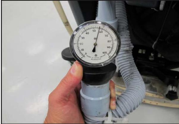
3. Install a one inch open-hole adapter between the hose end and the vacuum gauge.
