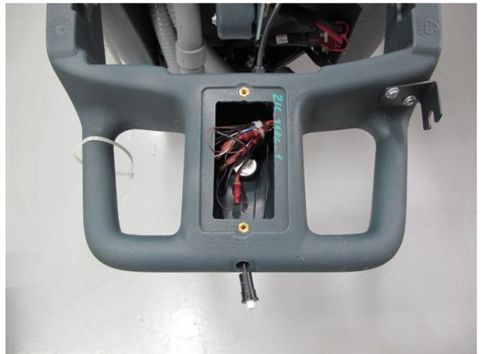
Handle Wiring Connections - ST models
