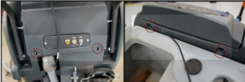
6. Tip cover away from machine and disconnect the clear pressure sensor hose from the fitting at the solution tank. **DO NOT TRY TO DISCONNECT THE HOSE FROM THE CIRCUIT BOARD.**
