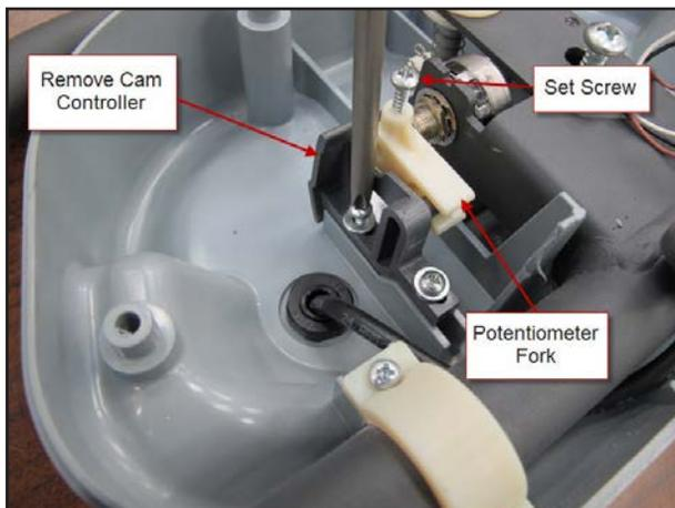
6. Loosen set screw and remove the potentiometer fork.
