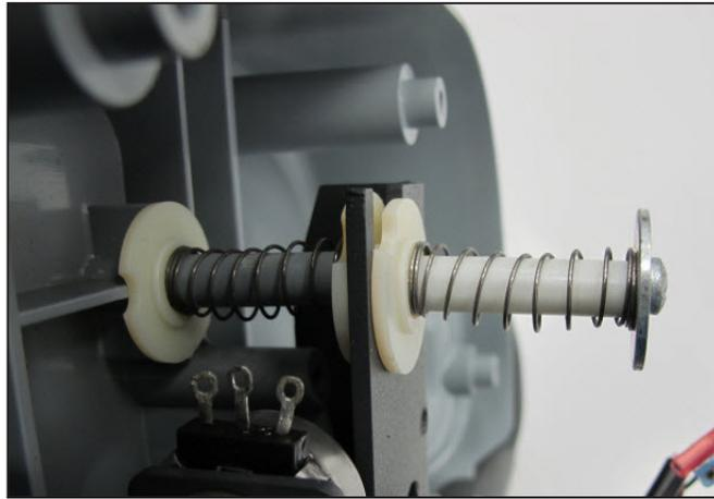
3. Next, prepare the upper stack for assembly as shown. Install it and tighten the screw. (Do not over-tighten the screw or it will strip out the tower).
