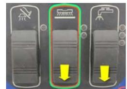
The red battery Indicator will remain on and the fault indicator will be flashing a numeric value that represents the current setting. To change the setting, press the solution switch forward to increase the value or backwards to decrease the value. To save the setting, press the scrub switch forward (All LEDs will turn on) then turn off the key switch.
