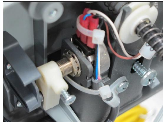
5. Remove the cam controller.
