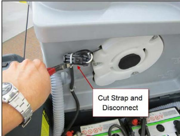
3. Remove vacuum motor cover mounting screws and cover. Note: The vacuum motor cooling fan guard may come off the end of the motor. Do not run the motor without the guard in place. Make sure that it is put back on during reassembly.
