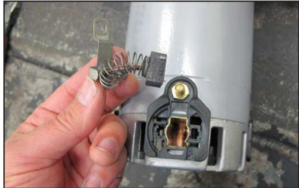
5. Reassemble in reverse order lining up the two locking tabs of the brush cap when installing the brush cap. Repeat for second carbon brush.
