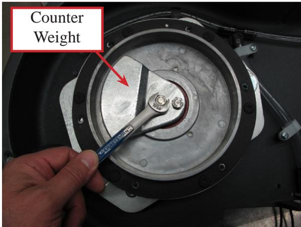
5. Lift the driver motor with the eccentric from the brush motor shaft being careful not to lose the square-cut key.
