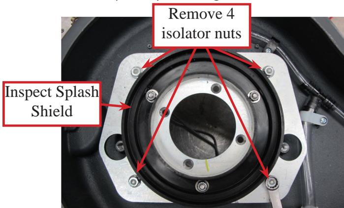
5. Inspect the splash shield and replace if damaged.
