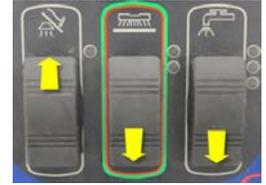
The Regular Scrub Pressure Indicator will remain on and the Fault Indicator will be flashing a numeric value that represents the current setting. To change the setting, press the solution switch forward to increase the value or backwards to decrease the value. To save the setting, press the scrub forward (All LEDs will turn on) then turn off the key switch.
