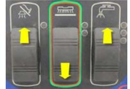
The Vacuum Indicator will remain on and the Fault Indicator will be flashing a numeric value that represents the current setting. To change the setting, press the solution switch forward to increase the value or backwards to decrease the value. To save the setting press the scrub switch forward (All LEDs will turn on) then turn off the key switch.
