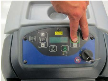
2. While holding both switches, turn the Key Switch to the ON position.
