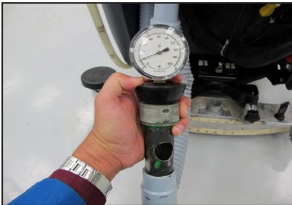
4. Turn the vacuum motor on and measure the vacuum. If it is within 10% of the specs, the vacuum system is working properly. If the reading is too low, check for a restriction in the system.
