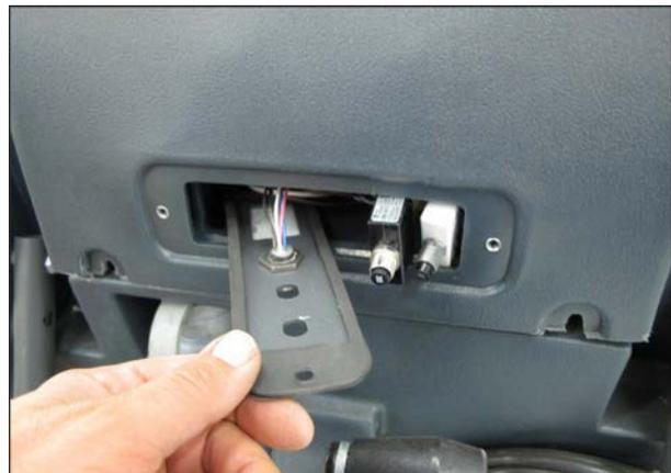
5. Remove electrical panel cover mounting screws.
