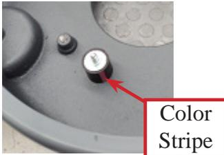
3. Apply Loctite blue 243 threadlocker or equivalent to the threads of each isolator. Install the motor plate and 4 isolator nuts. Torque each nut to 8-10 ft. lbs. (10.8- 13.5 N m). Ensure that the isolator rubber does not twist when you tighten the nuts. Visually inspect the color stripe to make sure that it is straight line and not twisted. If it is twisted, loosen the nut and repeat the procedure. It may be necessary to hold the isolator in position with your hand while tighten the nut.
