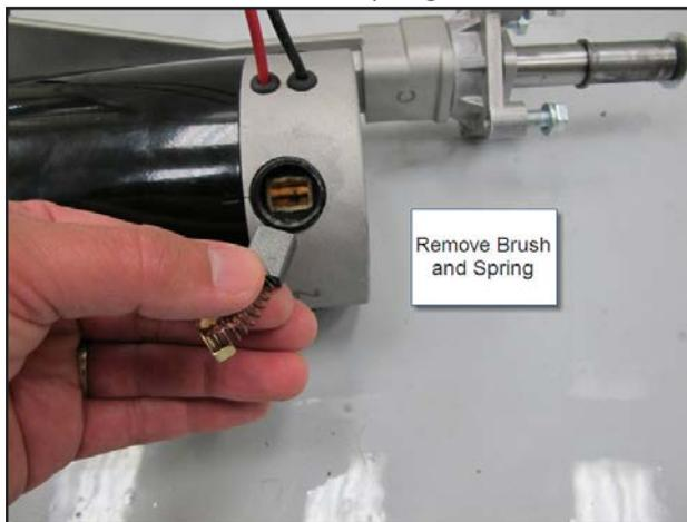
4. Install brush and spring. Install and tighten cap with a screwdriver.
