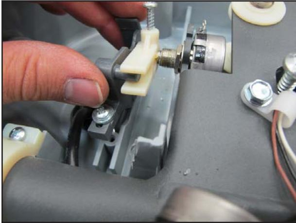
10. Install the cam controller inserting the pin end into the fork.
