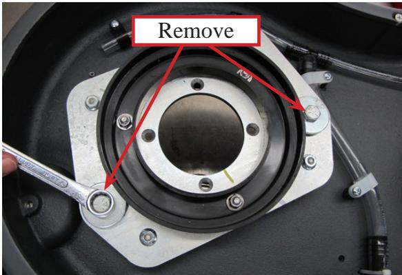
4. Remove the motor plate by removing the 4 isolator nuts.
