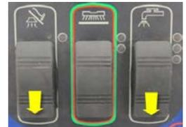
The green Battery Indicator will remain on and the fault indicator will be flashing a numeric value that represents the current setting. To change the setting, press the solution switch forward to increase the value or backwards to decrease the value. To save the setting, press the scrub switch forward (All LEDs will turn on) then turn off the key switch.
