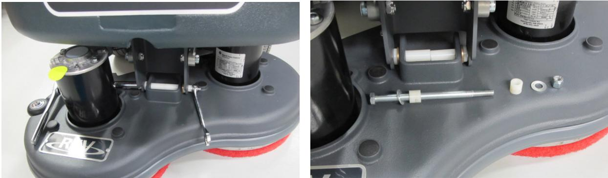
5. Carefully cut the tie straps around the brush motor wire loops. (Do not damage the wires)
