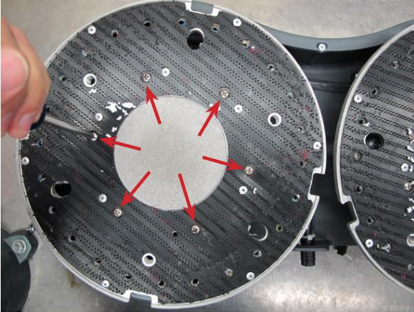
4. Remove the counter weight by removing the two attaching bolts.
