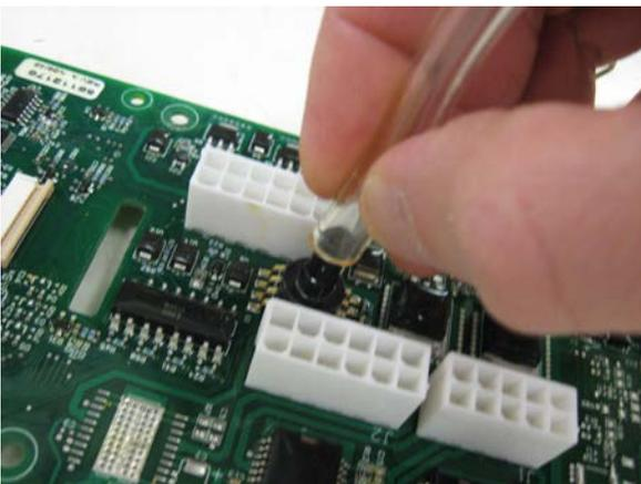
11. Reassemble in reverse order, taking care not to damage the printed circuit ribbons used to connect the circuit board to the control switch interface panel. If you did not drain the solution tank earlier, you must do so before connecting the pressure sensor hose in order for the solution level “gauge” to work properly.
