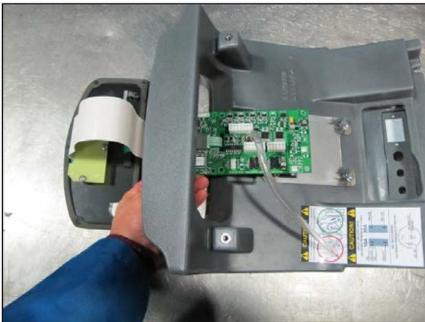
11. If the board is being replaced you will need to use a new pressure sensor tube or transfer the existing tube from the old board. Follow the steps below to transfer the tube.
