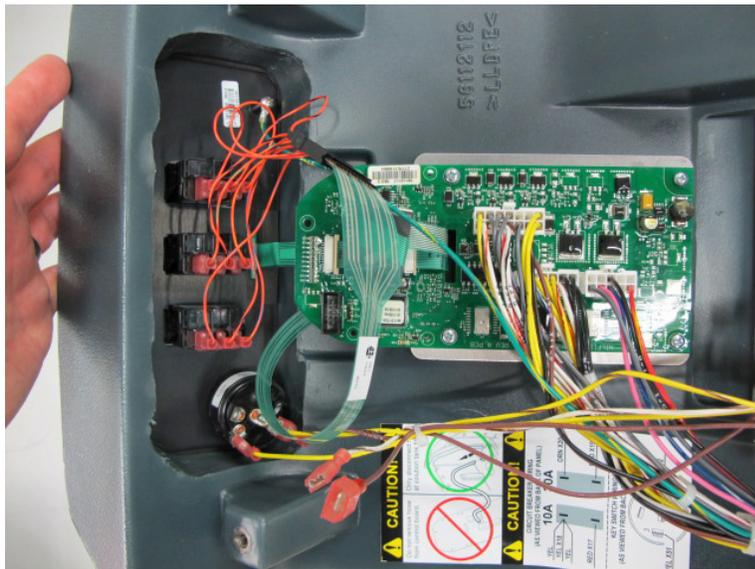
7. Place electrical panel cover on work bench. Disconnect the “ribbon” connector to the control switches. (Note the orientation of the ribbon to the wiring connector. )
