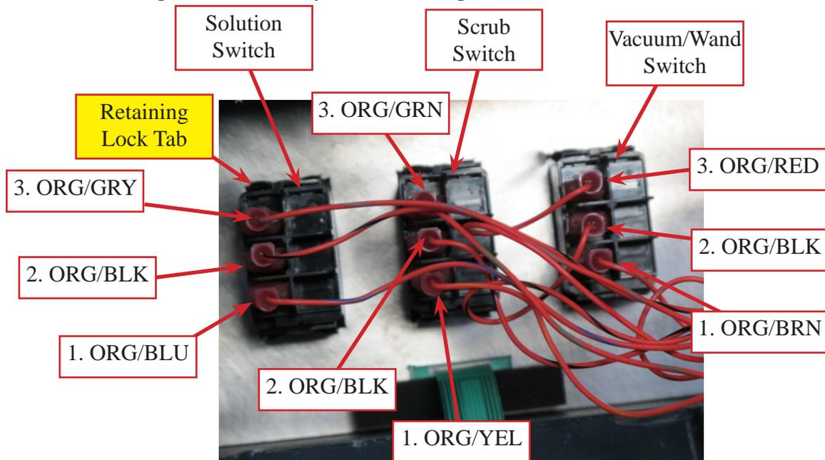
4. Push on the switch retaining lock tabs located at each corner and push the switch back through the cover.
