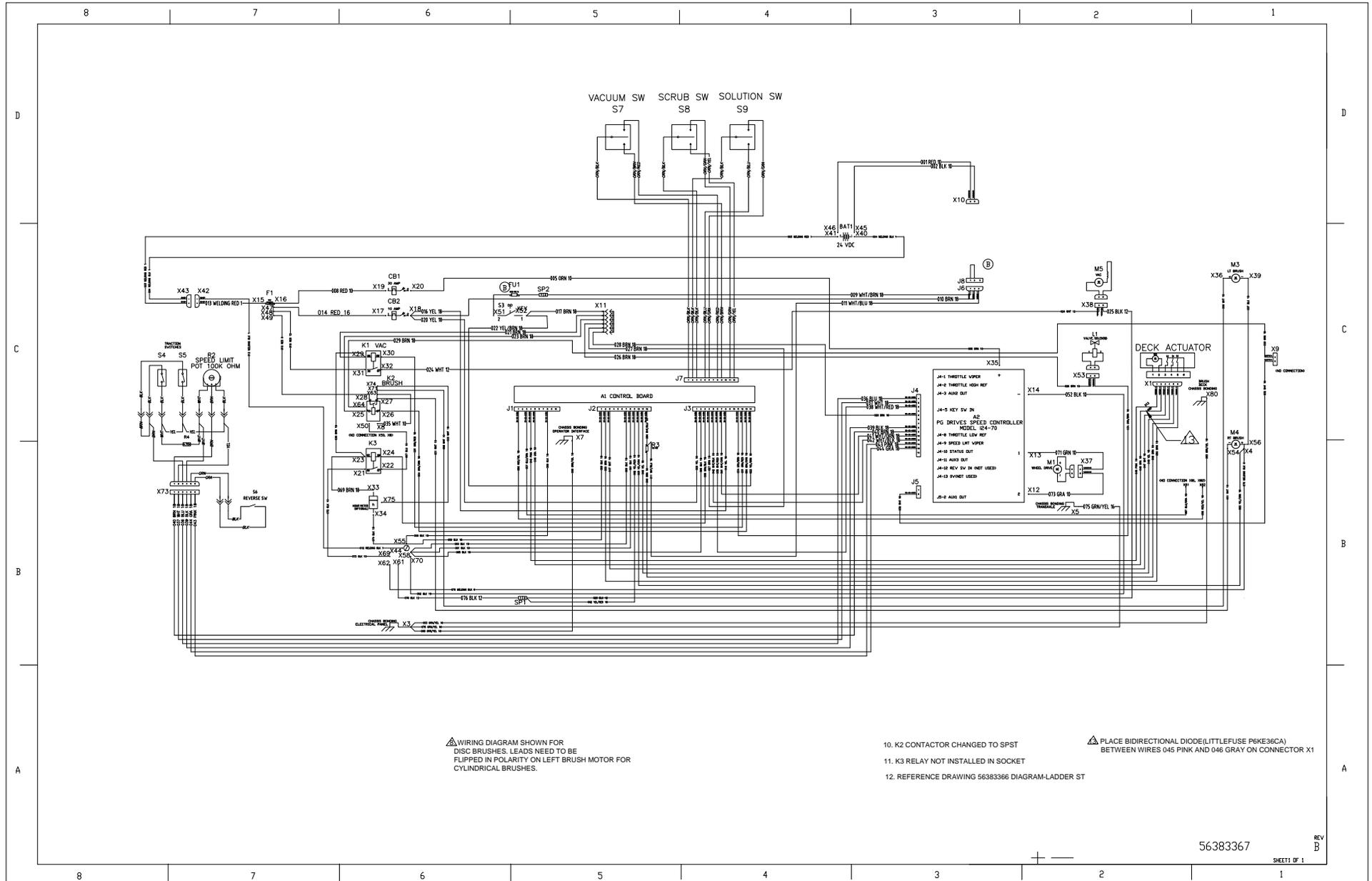
▲ WIRING DIAGRAM SHOWN FOR DISC BRUSHES. LEADS NEED TO BE FLIPPED IN POLARITY ON LEFT BRUSH MOTOR FOR CYLINDRICAL BRUSHES.
