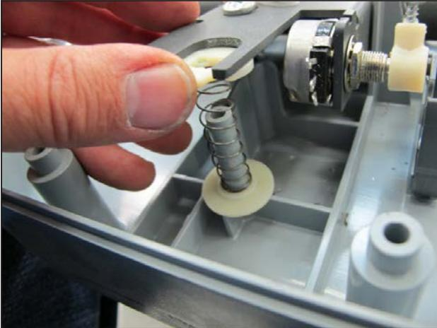
2. When reassembling, install the “lower stack” first. The shoulder of the nylon washers goes toward the spring. Carefully position the pieces so that they stay in place.
