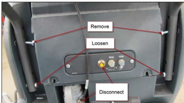
4. Remove circuit breaker mounting plate screws. Partially remove plate. Remove breakers from plate, then turn plate and insert into cover opening.
