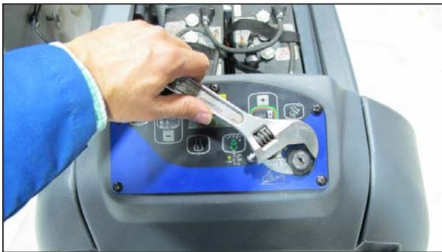
7. Remove electrical panel cover upper mounting screws.
