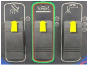
2. Wait approximately 3 seconds until all of the LEDs light up and then turn off. The low solution flow indicator light should remain on to confirm that you are in the service test mode.
