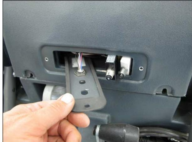
5. Remove electrical panel cover mounting screws.
