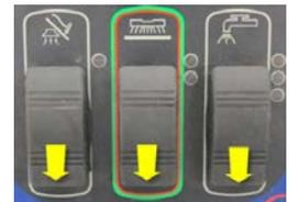
The Regular Scrub Pressure and Heavy Scrub Pressure Indicators will remain on and the fault indicator will be flashing a numeric value that represents the current setting. To change the setting, press the solution switch forward to increase the value or backwards to decrease the value. To save the setting, press the scrub switch forward (All LEDs will turn on) then turn off the key switch.
