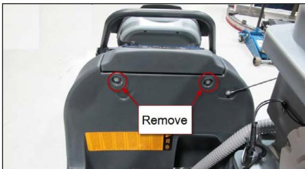
8. Loosen electrical panel cover lower mounting screws.
