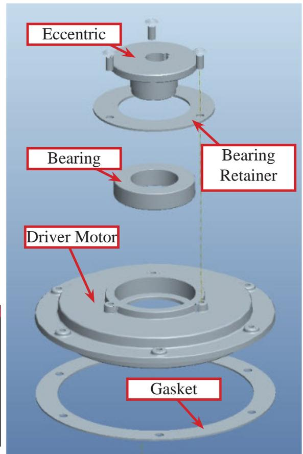
2. Press the bearing into the driver motor.
