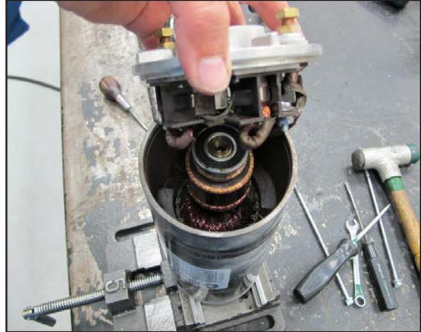
3. Remove the 2 through bolts and pry off the endplate assembly.
