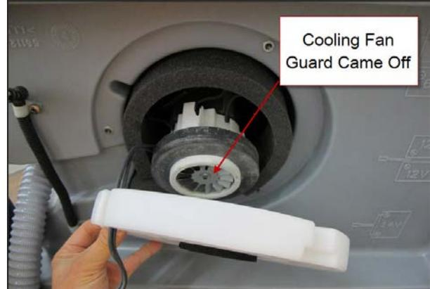
4. Remove vacuum motor and foam pieces. Pay attention to how the foam pieces are positioned.
