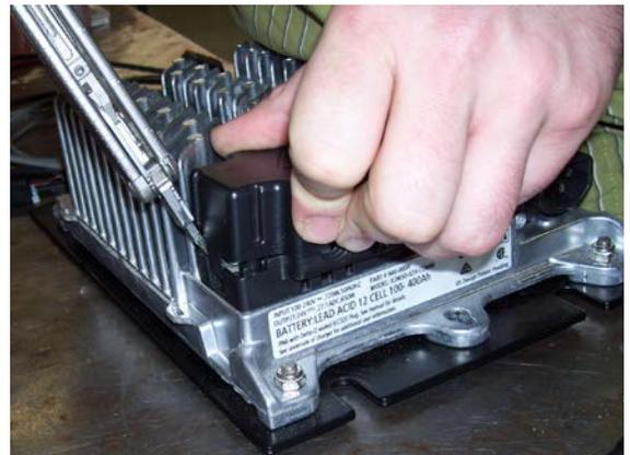
6. Remove the clamp (C). Disconnect the battery positive and negative wires (6) and the interlock wire (7)
