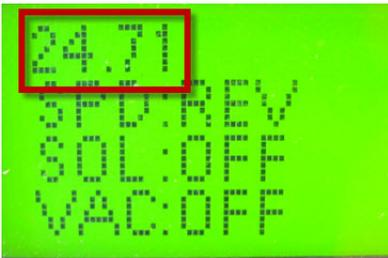
**Speed Control Forward/Reverse Signal AND Reverse Signal** – The Main Machine controller interprets these two signals that it receives from the Drive Motor Controller and displays the information on the LCD.
