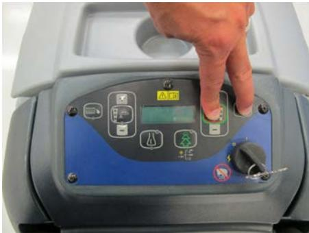
2. While holding both switches, turn the main power key switch to the on position.
