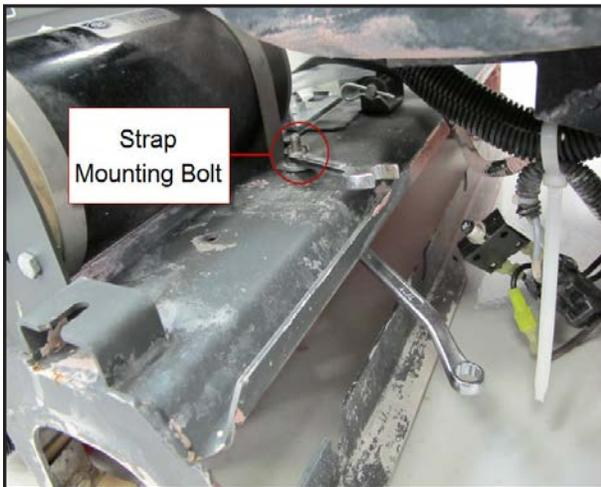
9. Remove the motor end mounting bolts.
