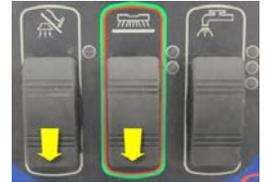
The yellow Battery Indicator will remain on and the fault indicator will be flashing a numeric value that represents the current setting. To change the setting, press the solution switch forward to increase the value or backwards to decrease the value. To save the setting, press the scrub switch forward (All LEDs will turn on) then turn off the key switch.
