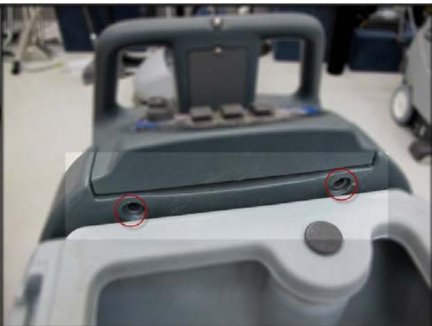
6. Tip cover away from machine and disconnect electrical connectors from the Main Machine Controller and Key Switch. Remove the control switch interface panel ground screw.
