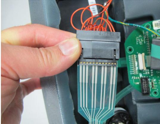
3. Disconnect the wiring from the switch you are removing.
