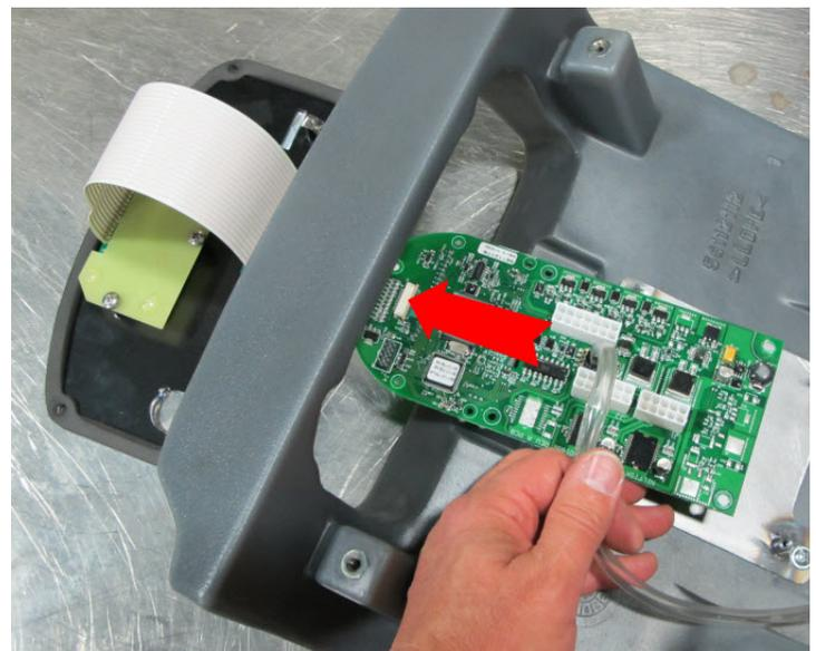
10. If the board is being replaced you will need to use a new pressure sensor tube or transfer the existing tube from the old board. Follow the steps below to transfer the tube.
