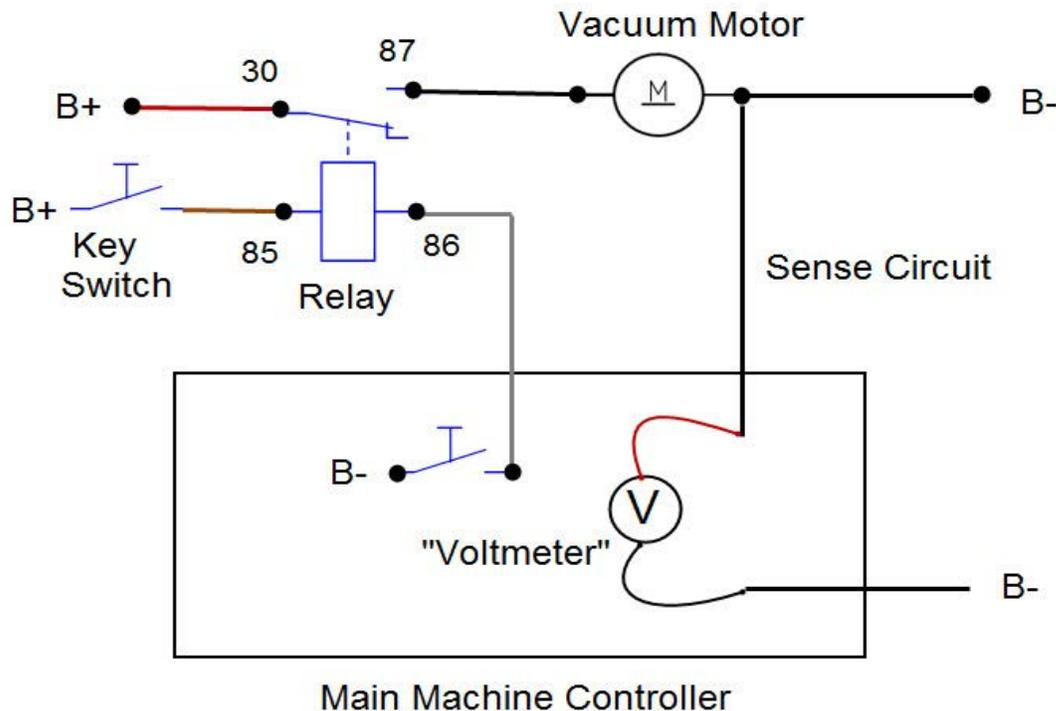
The vacuum contactor (relay) is turned on when the following inputs are met:
