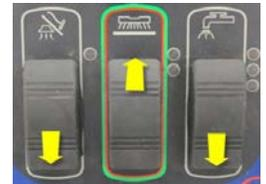
The High Solution Flow Indicator will remain on and the Fault Indicator will be flashing out all historical codes set since the last time they were cleared. To exit this function without clearing codes, press the scrub switch forward. To clear historical codes press the solution switch forward.
