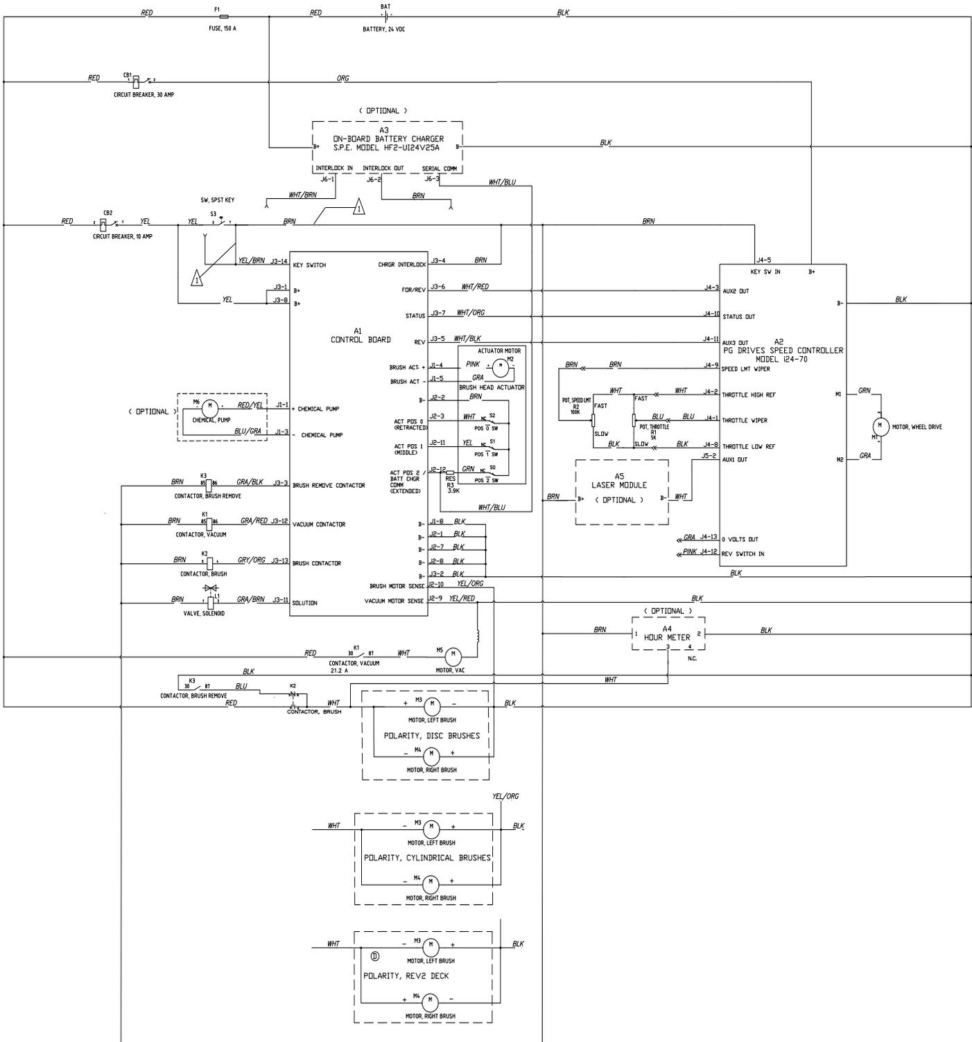
⚠ WHEN ON BOARD CHARGER IS USED , REMOVE BRN WIRE FROM KEY SW. CONNECT TO BRN WIRE FROM BATTERY CHARGER & REPLACE WITH WHT/ BRN FROM CHARGER. ALSO MOVE YEL/BRN WIRE AT KEY SWITCH FROM BRN TO YEL
