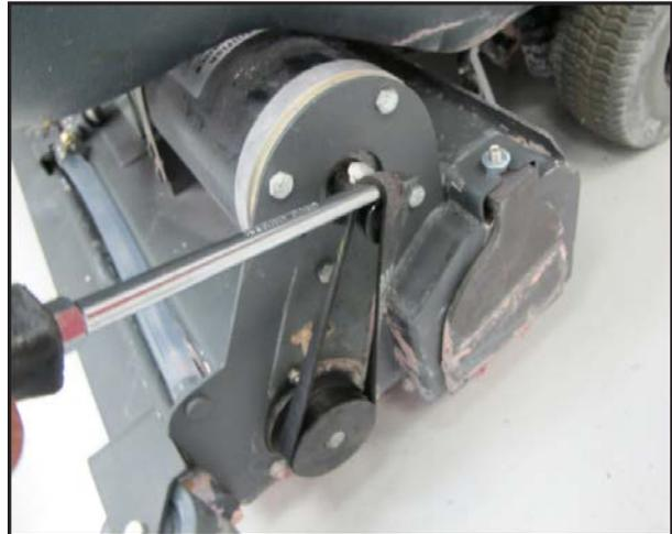
5. If the belt grooves are not quite in place, push on the side of the belt while rotating the pulley until the belt grooves are properly seated in the pulley.
