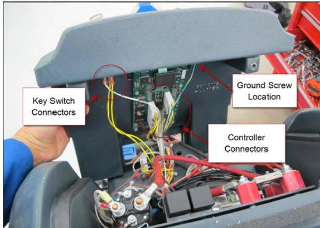
8. Remove the electrical panel cover and place on a work bench.
