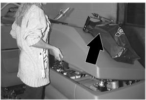
4. Check the water level in all the battery cells.
