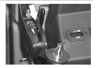
5. Push the pinch valve closed by hand. With the pinch valve in the closed position, tighten down on the cable swivel.
