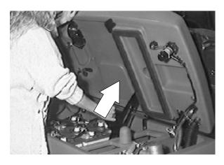
4. Align the top hole in the prop rod with the hole in the solution tank. Reinstall the M8 hex screw, sleeve, and washer. Tighten to 18 – 24 Nm (15 – 20 ft lb).
