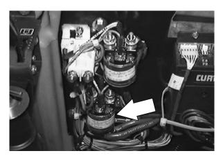
6. Reconnect the wire harness to the power contactor. See the electrical schematic in this section.
