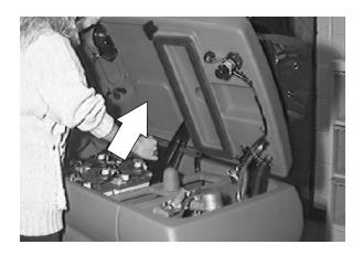
Remove the scrub brush from the motor that the belt needs to be changed. See TO REPLACE A CYLINDRICAL SCRUB BRUSH instructions in this section.
