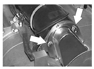
Loosen the M8 hex nut on the belt tension bolt under the motor. Turn the tension bolt down far enough to slip the belt off the pulley.
