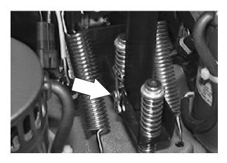
9. Remove the clevis pin and the roller from the scrub head roller guide bracket.
