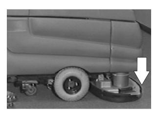
3. Raise the solution tank until the prop rod is engaged.
