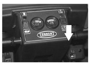
Reinstall the shroud locking bracket to the adjustable handle assembly. Reinstall the M8 hex nut and star washer. Tighten to 12 - 16 Nm (9 - 12 ft lb).
