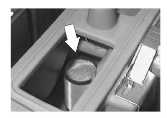
A vacuum fan filter is located in the recovery tank, for machines serial number 006956 and above. Remove and clean this filter daily. Clean by shaking dust or rinsing pleats with low pressure water. For machines below serial number 006956, a screen is located in the solution tank.
