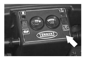
The optional 5700 XP instrument panel consists of a circuit board, a touch panel, and a water/dust resistant plastic enclosure. Its touch panel controls various machine functions, while its indicator lights keep the operator informed on the machine performance.
