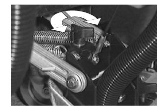
5. Raise and lower the squeegee blade again to check level with the floor.
