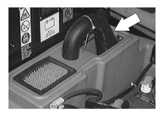
15. Remove the drain hoses from the back of the recovery tank.
