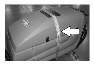
The rear tie-down locations are on either side of the machine frame by the rear casters.
