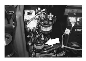
3. Disconnect the wire harness from the power contactor.
