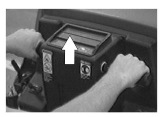
6. Remove the two M3 flat head screws holding the shield plate to the adjustable handle assembly. Remove the shield plate.
