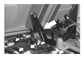
Open and close the valve handle. Check to make sure the pinch valve is properly controlling the solution flow.
