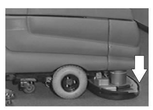
3. Raise the solution tank and engage the prop rod.
