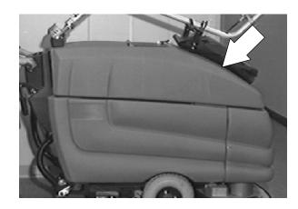
6. Disconnect the battery connector from the machine connector.
