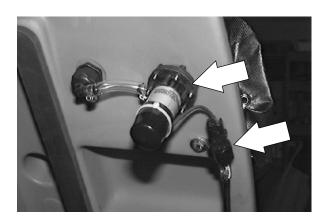
6. If the machine is equipped with ES™, disconnect the hose coming from the pump and going to the front of the tank. Loosen the collet at the tank and pull the hose out.
