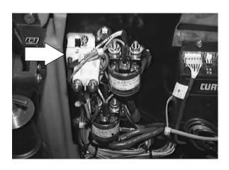
3. Disconnect the wire harness from the SPST contactor.
