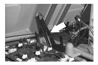
3. Loosen the swivel on the cable at the water valve end.
