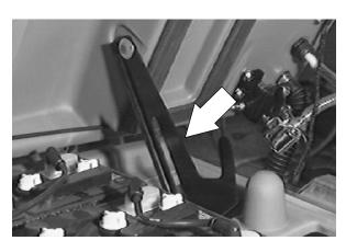
4. Remove the four M8 hex screws holding the front cover to the machine. Remove the cover.
