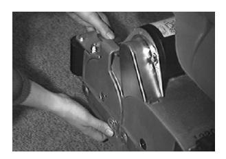
9. If the brush patterns are not both  $40 \pm 5$  mm  $(1.5 \pm 0.25$  in) wide, then use a 17mm wrench on the M10 hex screw, located on the pivot bracket, to adjust the angle of the scrub head. Make sure to re-tighten the M10 jam nut.
