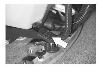
3. Block the machine tires that are not being jacked up, to secure the machine position.
