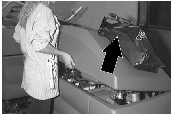
4. Check the water level in all the battery cells.
