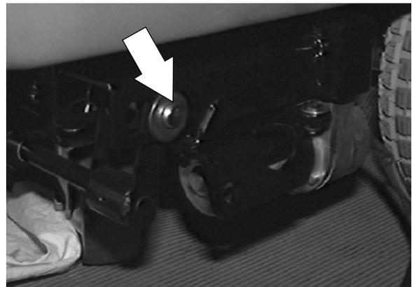
4. Remove the three M8 hex screws holding the actuator mounting bracket to the machine. Remove the mount bracket from the machine with the actuator inside it.
