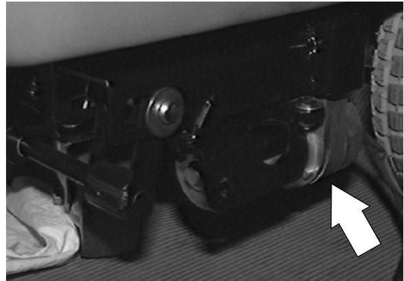
3. Remove the two hair pins and two clevis pins holding the squeegee lift actuator to the mounting bracket.
