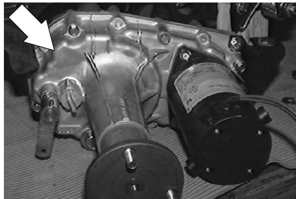
3. After the transaxle is removed from the machine, place it in a large vice with the drive motor facing up.
