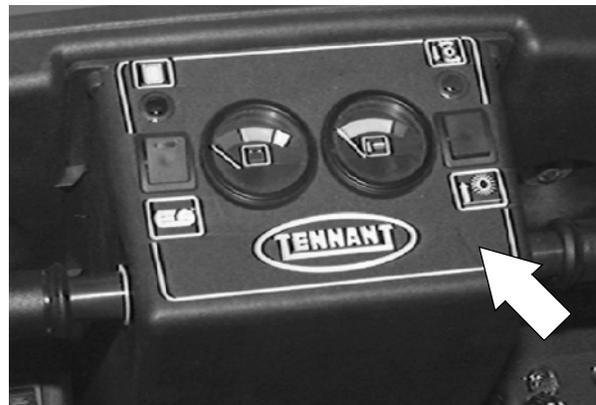
The optional 5700 XP instrument panel consists of a circuit board, a touch panel, and a water/dust resistant plastic enclosure. Its touch panel controls various machine functions, while its indicator lights keep the operator informed on the machine performance.
