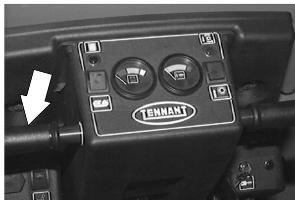
4. Remove the M6 hex screw and nyloc nut holding the white plastic speed control gear to the steering handle.
