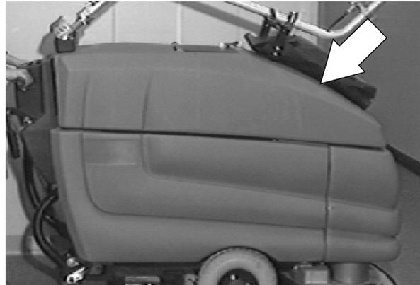
2. Align the two hinges with the threaded inserts in the tank. Install the two M8 flat head screws and tighten to 18 - 24 Nm (15 - 20 ft lb).
