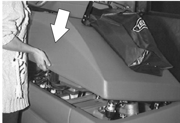
10. Remove the two M8 flat head screws holding the hinges to the outside of the solution tank.
