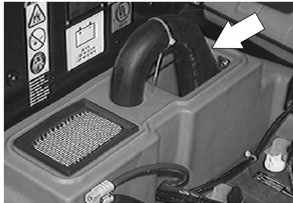
15. Remove the drain hoses from the back of the recovery tank.
