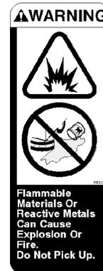
**FLAMMABLE SPILLS LABEL - LOCATED THE OPERATOR CONSOLE.**
