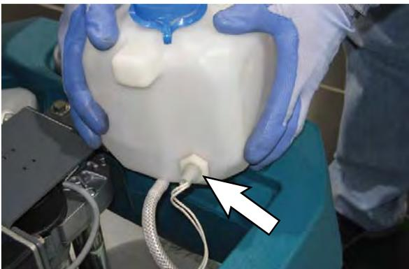
6. Reinstall the liquid level sensor in reverse order of disassembly.
