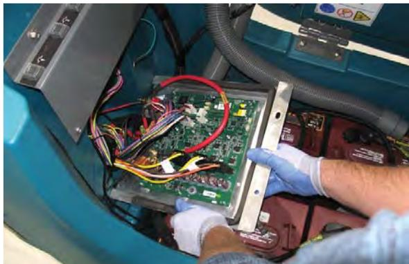
*NOTE: To avoid damaging electronic components, a static ground strap must be worn at all times while handling circuit boards / control modules. Attach the other end of the static ground strap to the machine chassis.*
