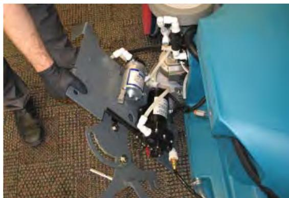
10. Disconnect the main wire harness from the pump.
