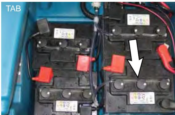
4. Replace damaged / worn fittings, hoses, and battery caps as necessary.
