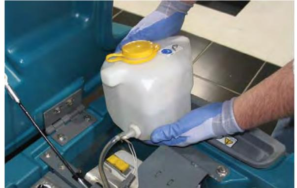
9. If necessary empty the solution from the tank.
