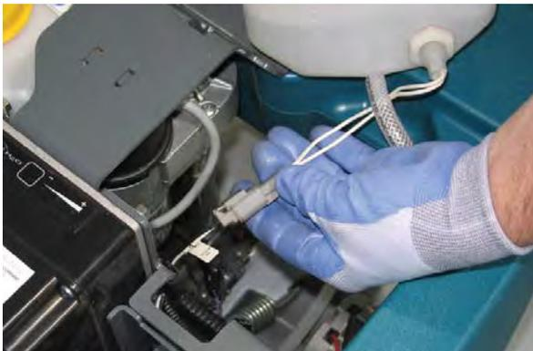
5. Remove the liquid level sensor from the tank.
