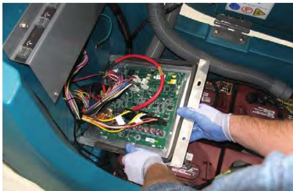
6. Disconnect all cables connections from the circuit board.
