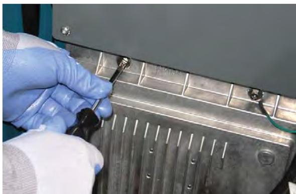
*NOTE: To avoid damaging electronic components, a static ground strap must be worn at all times while handling circuit boards / control modules. Attach the other end of the static ground strap to the machine chassis.*
