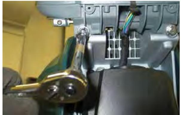
9. Lift up and forward to remove the operator console from the machine.
