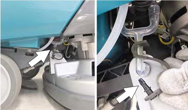
6. After storing machine in freezing temperatures, drain any remaining antifreeze from the solution tank and from the optional Severe Environment detergent tank. Add clean water to solution tank and to optional detergent tank and operate the machine to flush system.
