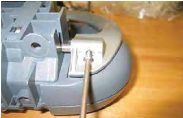
14. Release the bail return spring, rotate the bail handle shaft toward the bottom of the operator console, and slide the bail handle shaft to the side to remove.
