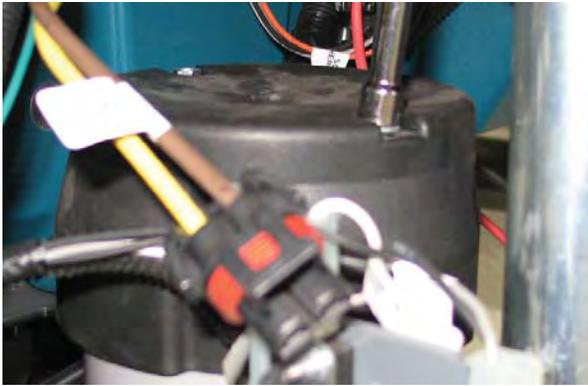
5. Remove the pan screw and spring clip securing the carbon inside the motor and carefully pull the carbon brush assembly from the brush motor.
