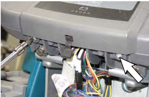
5. Lift up on the bottom of the panel and slide downward to remove.
