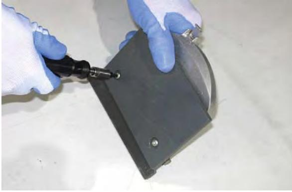
14. Adjust the brush taper. Turn the idler plug clockwise to increase the taper at that end of the brush and counterclockwise to decrease the taper at that end of the brush.
