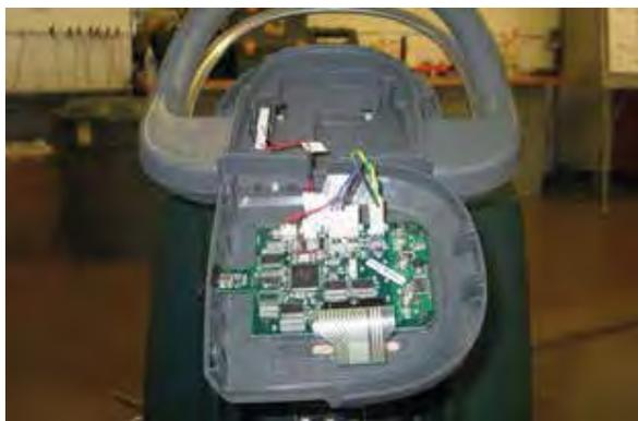
6. Disconnect all electrical connections from the interface module.
