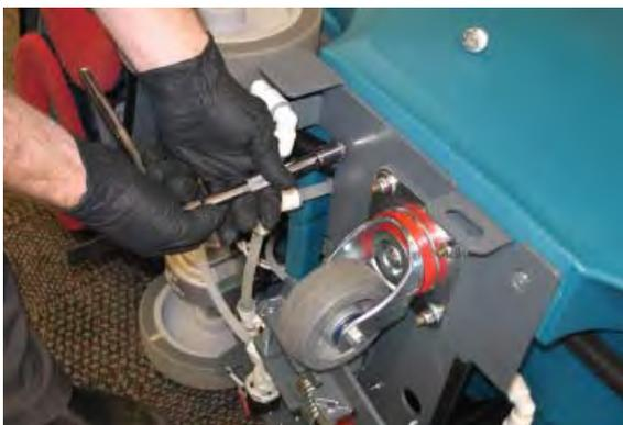
9. Carefully pull the rear frame from the machine.
