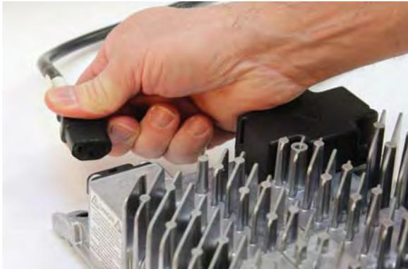
2. While reconnecting AC input, press and hold the Select Charge Profile Button for approximately 10 seconds, through the light check function, until the Error Indicator is illuminated (amber) and Battery Charging Indicator starts flashing (green).
