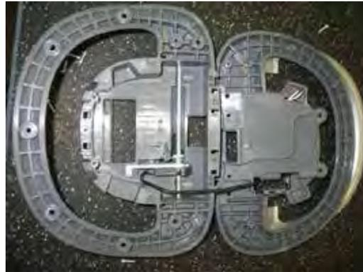
11. Remove the bail handle from the bottom control housing.
