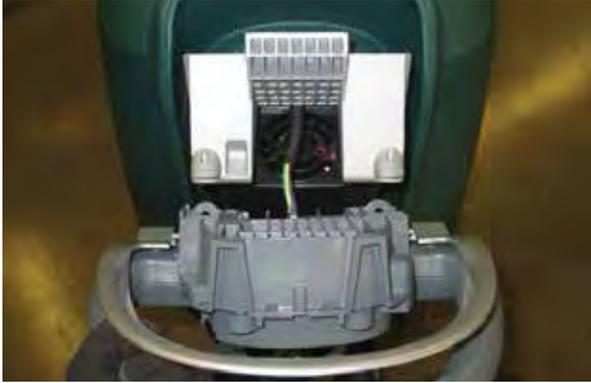
12. Remove the self tap screws from the front of the operator console.
