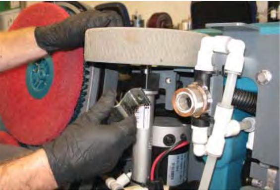
11. If replacing the transaxle assembly only: Remove both wheels from the transaxle motor. Set the wheels, both keys, flat washers, and hex nuts aside. Discard the removed transaxle.
