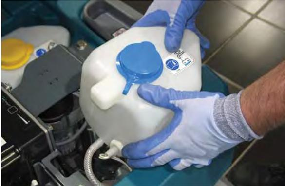
3. If necessary empty the solution from the tank.
