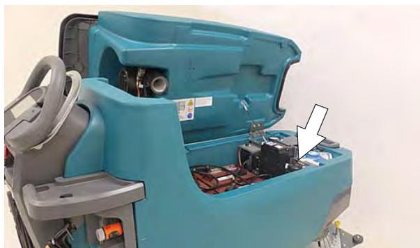
3. Disconnect the two hose connectors from the top of the cartridge by pressing the gray collars inward and pulling the connectors outward. Lift cartridge to remove.
