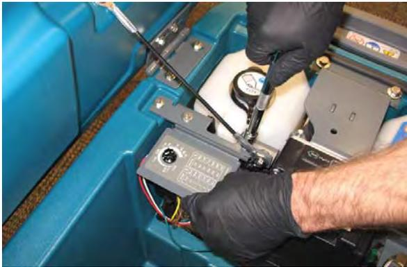
4. Carefully remove the detergent pump bracket / detergent pump assembly from the machine.
