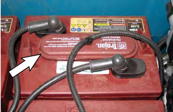
4. Replace the vent cap if it still leaks after tightening.
