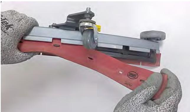
4. Rotate the rear blade to a new wiping edge and Reinstall blade. Make sure to align the slots in the blade with retainer tabs.
