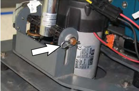
8. Remove the hex screws and flat washers securing the head lift bracket to the scrub head.
