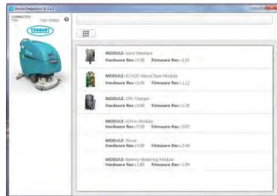
8. The Service Diagnostic tool may prompt to cycle the key switch OFF/ON during the process. If prompted, click the OK button and then cycle the key switch to allow the programming to continue.
