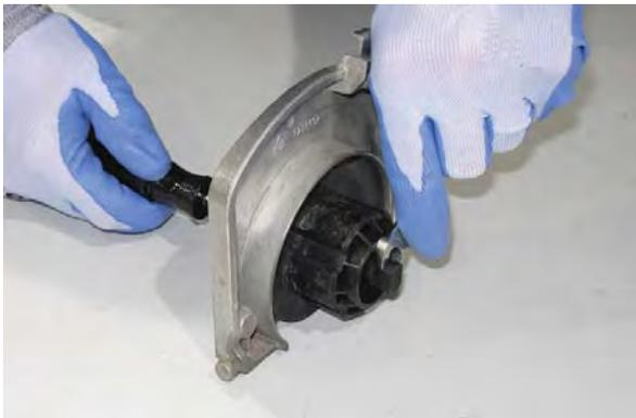
15. Reinstall the skirt cover onto the idler plate and reinstall the idler plate assembly onto the scrub head.
