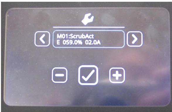
**M02: Scrub Motor 1:** Press the - (minus) button to set the actuator in the retract direction and the + (plus) button to set the actuator in the extend direction. Squeeze the bail to move the actuator. Press the check box to turn scrub motor 1 on or off. Displays the average voltage, PWM duty cycle, and motor current.
