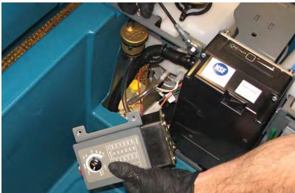
5. If replacing detergent pump assembly, remove the pan screws securing the detergent pump assembly to the detergent pump bracket.
