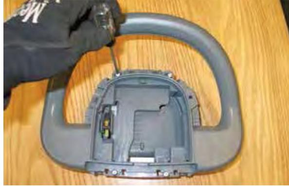
10. Remove the speed range dial and set aside. If replacing the potentiometer or directional switch, remove the nut securing the potentiometer or directional switch.
