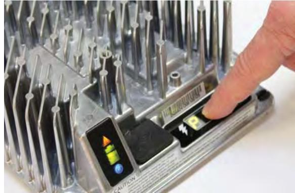
4. When the new charging profile is displayed, press and hold the Select Charge Profile button for 10 seconds to confirm selection and exit Profile Selection Mode. When the charge profile is confirmed, the Error Indicator and Battery Charging Indicator lights will turn off and the blue AC Power Indicator will remain illuminated. Release the Select Charge Profile button.
