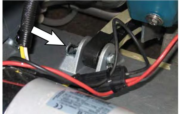
13. Remove the clevis pin and cotter pin securing the scrub head pivot to the head guide bracket.
