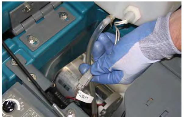
11. Remove the liquid level sensor from the tank.
