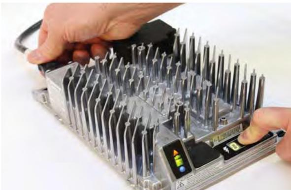
3. Press and release the Select Charge Profile Button to advance through the charge profiles. The selected charging profile will be displayed up to three times.
