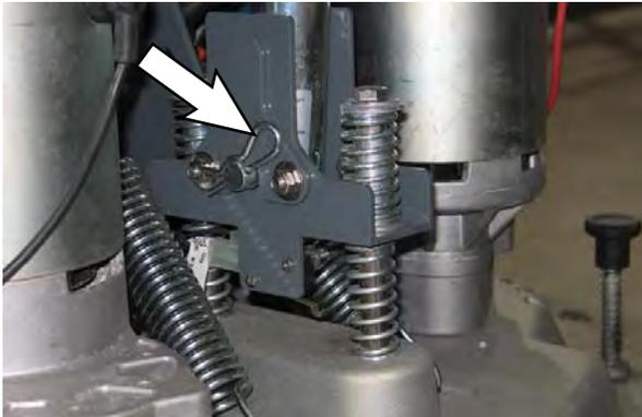
10. Remove the cotter pins and clevis pins securing the head lift arms to the scrub head assembly.
