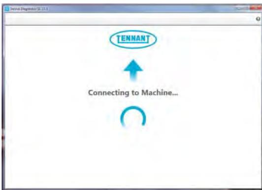
5. The Service Diagnostics tool automatically detects a new interface module installation. Enter the model and serial number and then click the arrow button.
