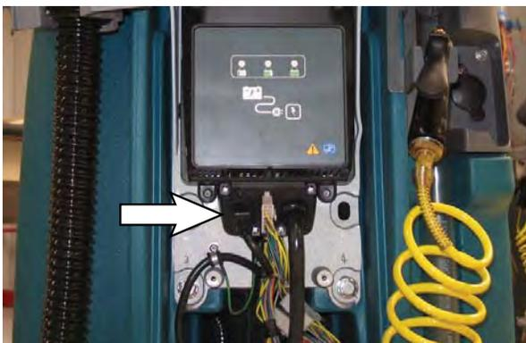
5. Remove the on-board battery charger from the machine.
