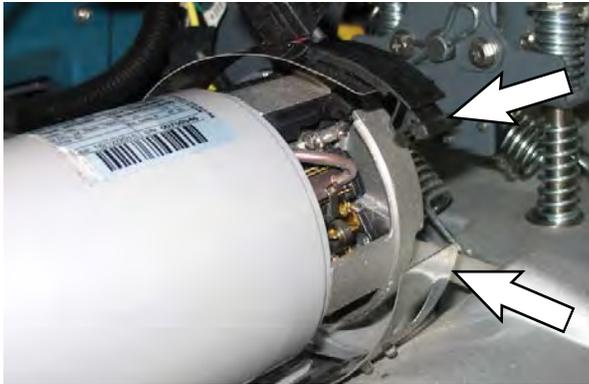
4. Carefully pull the carbon brush from the cylindrical brush motor.
