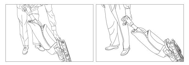
If you would like to load the i-mop into a vehicle or lift it over obstacles, always use two hands. With one hand, hold the pole/handle, and with the other hand, lift the scrub deck.
