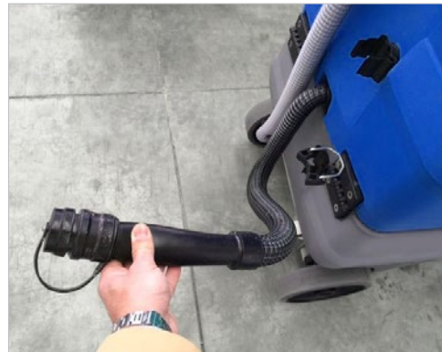
Dirty water drain hose
