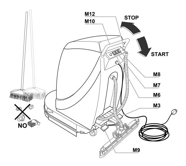
The area to be scrubbed: Debris and grit must be swept up before starting the scubbing operation to avoid vacuum line blockage and to permit the detergent to perform efficiently.
