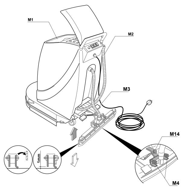
**Solution Tank:** The solution tank is located under the lid, at the front of the machine, with the filling-funnel **M1** in an accessible position for easy re-filling.
