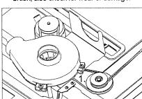
Check tension, wear and damages on the V-belt of the sweep roller drive.
