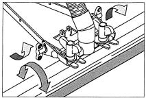
→ Tighten the wing nuts.
