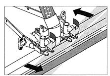
> Tighten the wing nuts.
