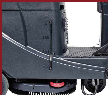
Water solution level indicator with volume visible on the tank
