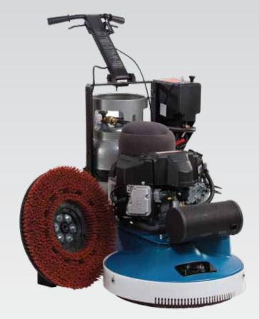
The Pride 2100 strip/buffer, offers two pieces of equipment in one. By simply changing one belt, this amazing floor care machine can buff at 2100 RPM's or strip at 500-700 RPM's. A 3600 floating, swivel, spin-on pad driver makes for easy maintenance. Run time is 5 to 6 hours per propane cylinder. Emissions protected by three-way catalytic muffler on Kawasaki Engine.
