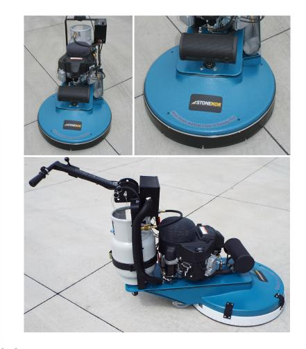
Stonekor's Dust Control Series is ideal for keeping a clean work area by actively capturing up to 95% of dust particles.
