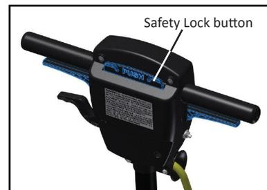
Once you have the handle height set to your preference and you are in the operators position, press in on the Safety Lock button with your thumbs and start the machine by depressing either the left, right or preferably both switch levers. Begin moving forward in straight lines. Check your pad every 15 to 30 minutes (depending on pad in use) to maintain optimum performance.
