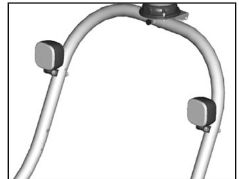
Movable working lights
