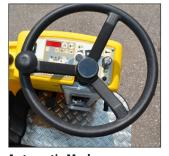
**Automatic Mode** Automatic mode starts all necessary operations of the scrubber once it is turned on, making operation effortless.
