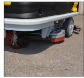
**Integrated Bumper** Integrated bumper keeps walls and other sensitive areas from being damaged.
