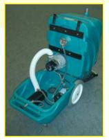
Unique clamshell design of the 1120/1160 models allows easy access to major working components.
