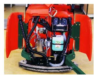
Direct access to all important parts and systems thanks to covers which can be opened for service and maintenance purposes. Pictured above for example, chemical metering system and dirty water recycling system.
