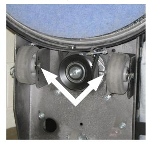
**NOTE:** To increase pad pressure (more aggressive) move wheels to rear of machine. To decrease pad pressure (less aggressive) move wheels toward the front of machine.
