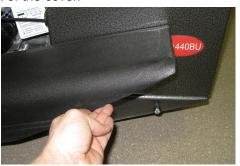
2. Pull the dust bag off the dust tube, keeping the closed end pulled downward to prevent spillage.
