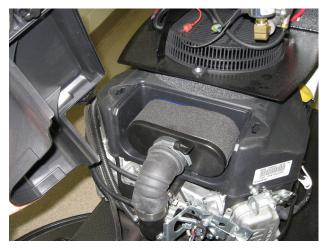
**CAUTION!** Do not wash the air cleaner filters. Do not oil the air filters. Do not use pressurized air to clean the air filters.
