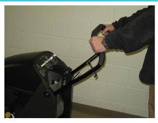
Do not try to start the machine with the bail throttle in the operating position.
