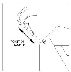
4. Tighten the handle pivotknobs.
