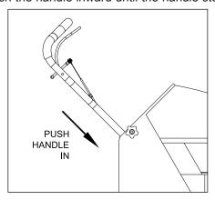
9. Tighten the handle pivot knobs on both sides of the bulkhead.
