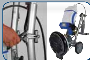
The Taz folds down to 30" tall which makes for easy transport and storage.
