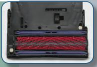
The cylindrical scrub brush has squeegee blades on either side for water pick in any direction. The squeegee blades can be raised to allow double scrubbing.
