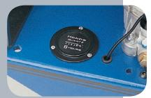
Lightning burnishers and stripper come with an hour meter to measure productivity and simplify scheduled maintenance.
