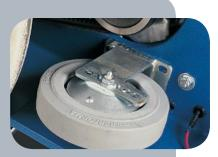
Wheel adjustment fine tunes pad pressure for maximum operator productivity.
