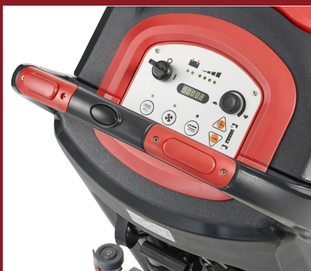
Control panel with intuitive display and buttons
