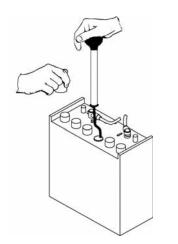
NOTE: Do not take readings immediately after adding distilled water, if the water and acid are not thoroughly mixed, the reading may not be accurate.
