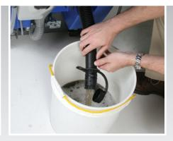
**Recovery tank draining** Convenient recovery tank dump hose.
