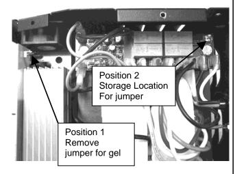
Configure the Charger for Flooded/AGM batteries
