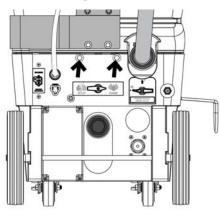
Installing metering tips for the Chemical feed system:
