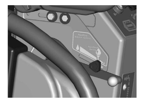
In order to consistently conserve water when using Aquastop brushes, the guide will stop the solution control lever at a low rate setting. This setting may be adjusted by loosening the knob, adjusting the lever, and retightening the knob. Slide the knob all the way forward to dispense maximum solution.
