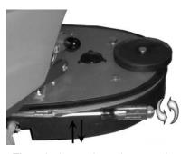
The splash guard may be moved up or down as the brush/pad wears by loosening the clamp on the back side of the deck with a flathead screwdriver or 9/ 32" (7mm) socket, then slide the splash guard to the desired height & retighten the clamp.
