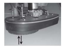
2. Brushes are installed/removed by hand. Push each brush up onto the hub until it "clicks". To remove, pull down on the edge of each brush.
