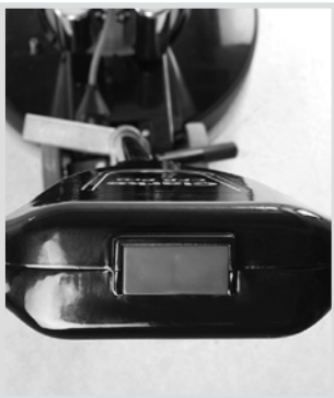
Safety lock-out switch.
