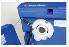
Quiet vacuum motor system - 65 decibels on disc, 63 decibels on the BOOST model. This allows the operator to use the scrubber in noise sensitive areas.
