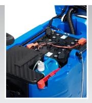
**Battery Compartment** The RA40<sup>™</sup> is available with wet or AGM maintenance-free batteries.
