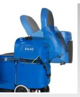
**Recovery Tank Access** Recovery tank fully tiltable gives easy access to battery compartment and the detergent container.
