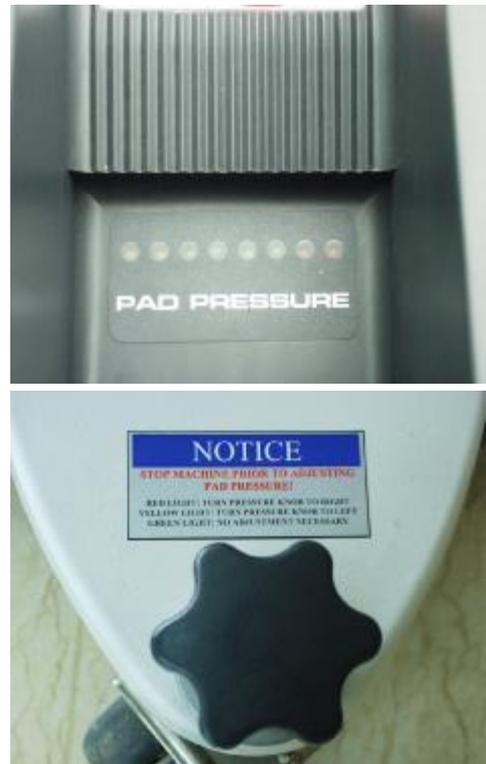
10] Once the machine has reached operating speed, look at the digital pad pressure meter located on the top of the motor cover. There are 3 light colors which will help you determine optimal pad pressure for operating the machine. RED LIGHT(S): If one or both red lights are illuminated, stop the machine and turn the pad pressure
