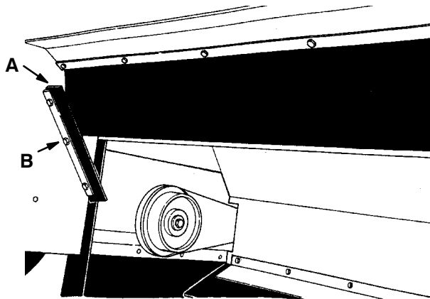
HOPPER SIDE SEALS A. Hopper Side Seal B. Seal Retaining Strip
