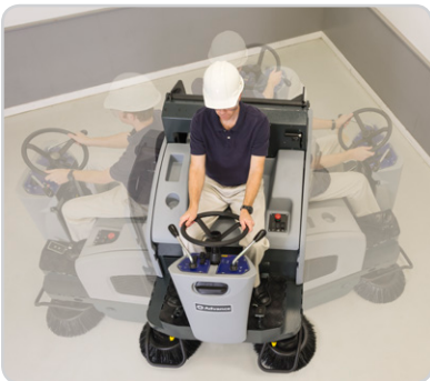
Front-wheel powered and steered drive wheel provides superior maneuverability, allowing operators to sweep in tight corners or narrow aisles.
