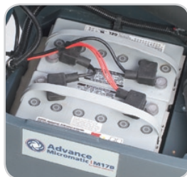
Maintenance-free gel batteries with onboard charger come standard on machine (M17B).
