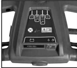
The SC350 offers four operating modes, including: off, water + brush, water + brush + vacuum, and vacuum only. Two adjustable flow rates—low and high—allow operators to easily match diverse application requirements.
