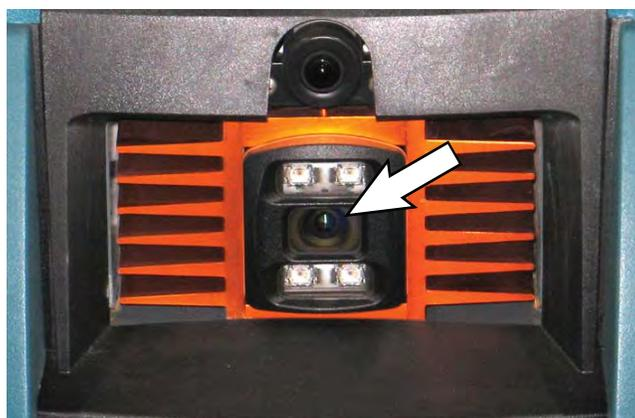
**REMOVE/REINSTALL/REPLACE THE FRONT 2D CAMERA**
