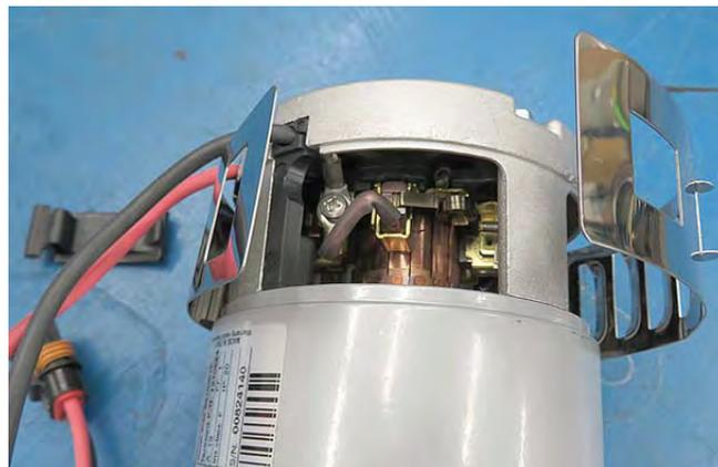
7. Lift the clip securing the carbon brush inside the scrub brush motor and pull the carbon brush from the retainer.
