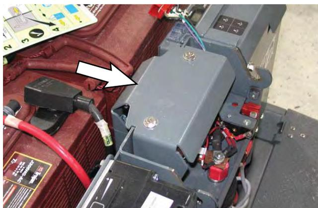
6. Disconnect wire harness connections from the top terminals of the contactor.
