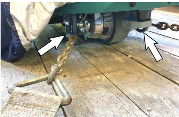
*NOTE: It may be necessary to install tie-down brackets to the floor of the trailer or truck.*
