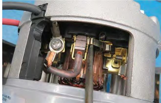
8. Remove the hardware securing the carbon brush cable to the scrub brush motor and remove the carbon brush from the motor.
