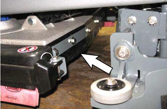
The skirts should clear the floor by 0 to 6 mm (0 to 0.25 in) when the scrub brushes are new and the scrub head is down.
