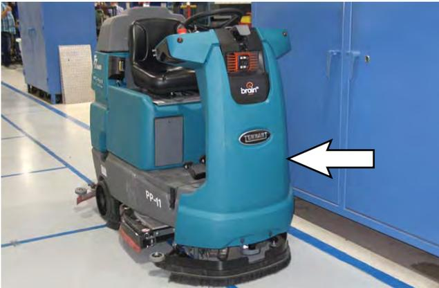
4. Remove the front bezel from the machine.
