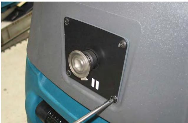
4. Carefully pull the blue start/pause button assembly from the recovery tank cover. Do Not break or damage wire/cable connections when pulling the blue start/pause button assembly from the recovery tank cover.
