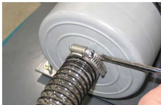
8. Remove the vacuum fan from the fan mounting bracket.
