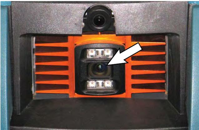
Side 2D and 3D cameras are located on each side of the machine.
