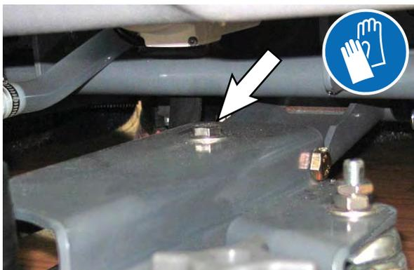
Turn the squeegee leveling bolt counter-clockwise to increase the deflection at the ends of the squeegee.
