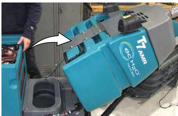
6. Remove the operator seat/seat plate from the machine.
