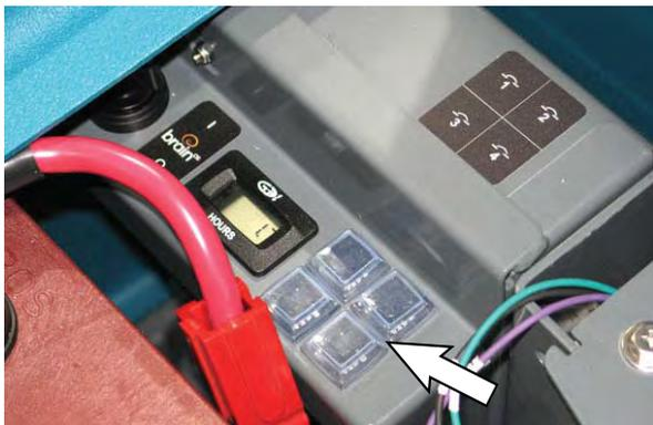
If the overload that caused the circuit breaker to trip is still there, the circuit breaker will continue to stop current flow until the problem is corrected.
