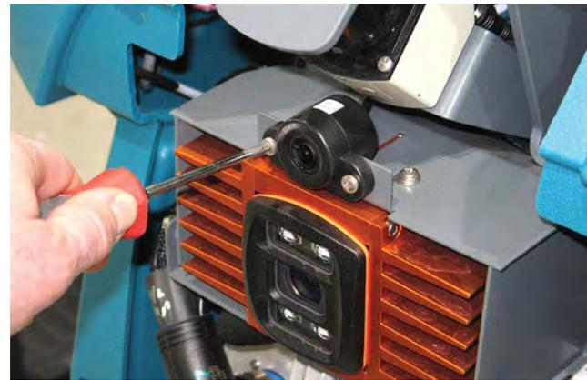
6. Disconnect the wire harness from the front 2D camera.
