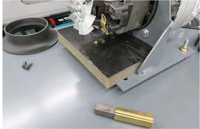
5. Inspect carbon brushes. Replace carbon brushes if they are stuck or are less than 10 mm (0.375 in) in length.
