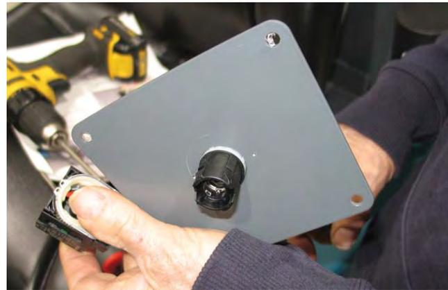
10. Install the new start/pause button assembly onto the start/pause button plate and tighten the retainer screw to secure the start/pause button assembly into place.
