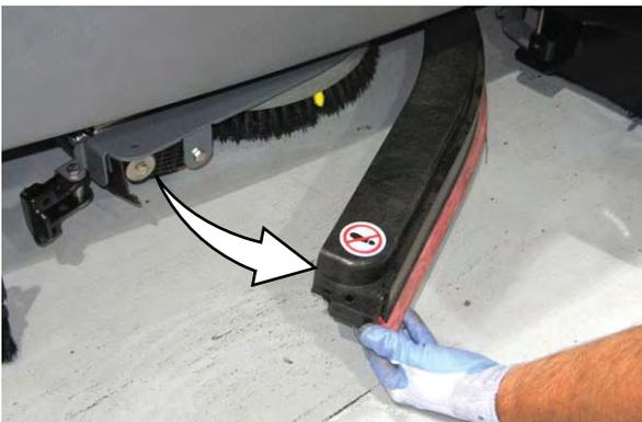
3. Pull the old side squeegee blade from the side squeegee retainer. Slide the new blade onto the retainer.
