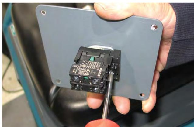
7. Press the retainer lever and remove the start/pause button assembly from the start/pause button plate.
