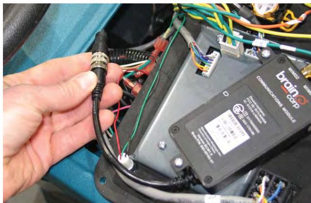
6. Remove the antenna/antenna bracket from inside the steering shroud.
