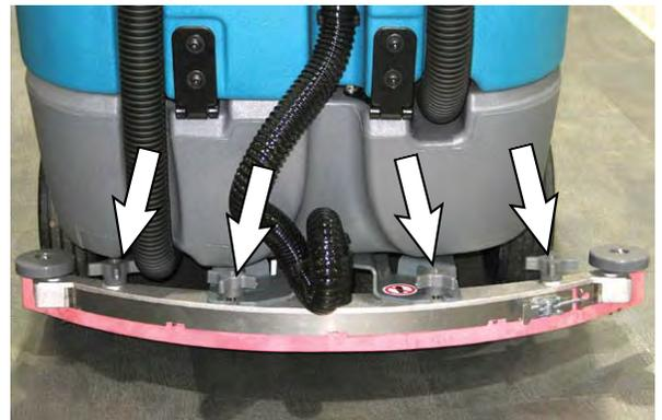
14. Reinstall the squeegee vacuum hose onto the rear squeegee assembly.
