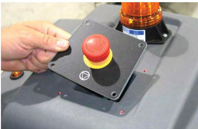
5. Push the lever to disconnect the E-Stop button connector from the E-Stop button.
