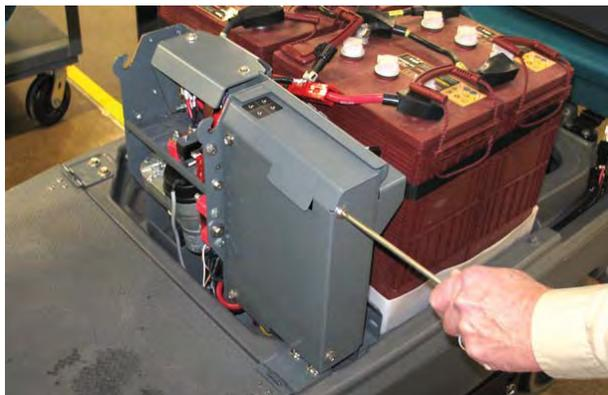
6. Disconnect all wire harness connections from the Kinetek controller.
