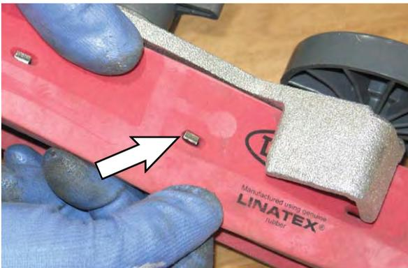
11. Reinstall the rear squeegee retaining band onto the squeegee assembly. Be sure each of the flanges on the retaining band are seated in the cut outs in the rear squeegee assembly.
