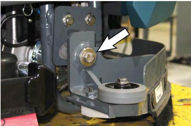
5. Pull the support bracket assembly from under the machine.
