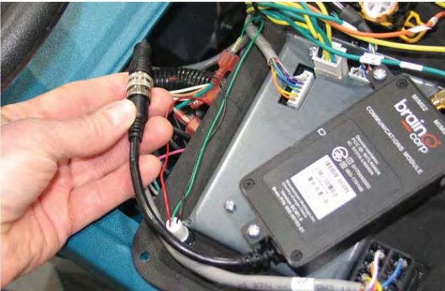
5. Disconnect the wire harness from the telemetry controller.
