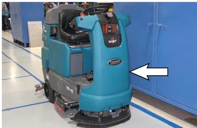
4. Remove the front bezel from the machine.
