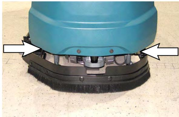
3. Position the machine at the loading edge of the truck or trailer.
