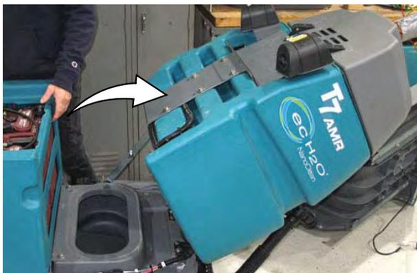
6. Remove the tank support bracket and tank support angle from the machine.
