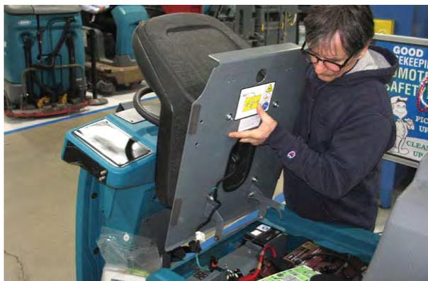
7. Remove the battery box cover from the machine.
