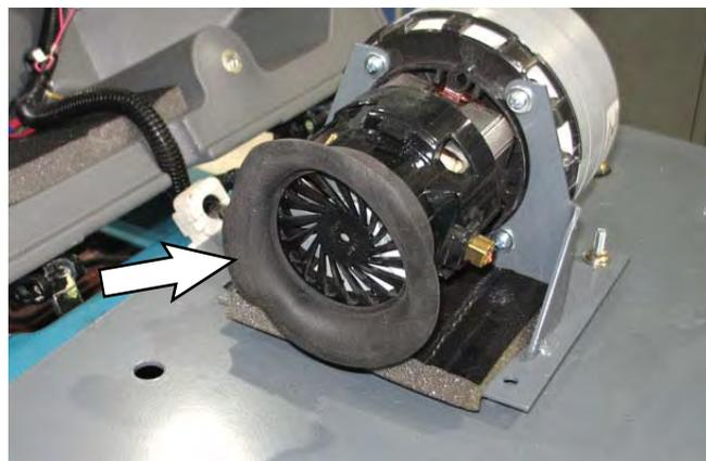
6. Disconnect the main wire harness from the vacuum fan.
