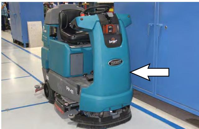
4. Remove the column access panel from the steering column. See FRONT COVERS GROUP.
