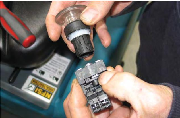
11. Connect the harness connections to the start/pause button assembly.
