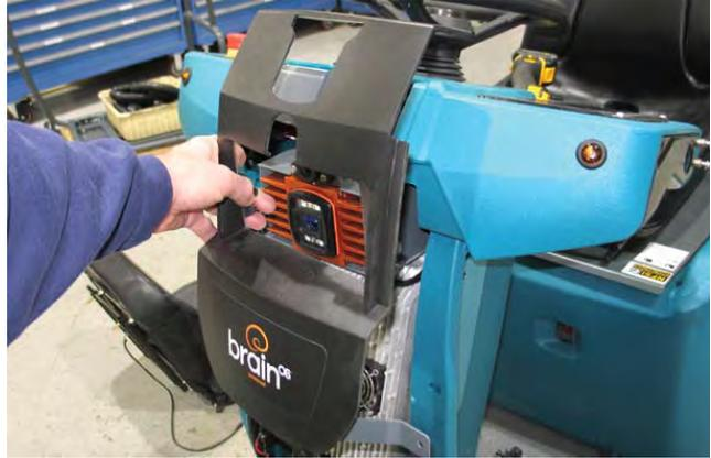
5. Remove the front 2D camera from the camera bracket.
