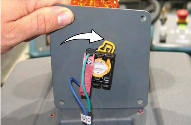
10. Push the lever to connect the e E-Stop button to the E-Stop button connector.
