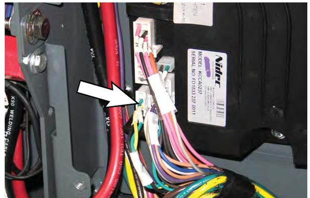
4. Connect the AMR SERVICE CONNECTOR to the service device.
