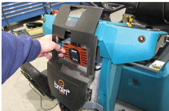
5. Disconnect all wire harness connections from the Brain controller.
