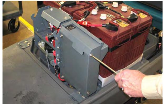
3. Disconnect the main wire harness SCRUB CONTROLLER connector from the Kinetek Control Module P4: CAN/Programming terminal.
