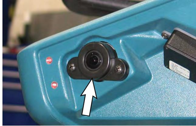
7. Install the new 2D camera into the steering shroud.
