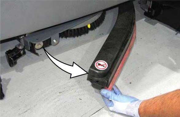
6. Press the spring clip together with the thumb and index finger. The brush/pad driver will drop off the drive hub. Remove the brush from under the machine.
