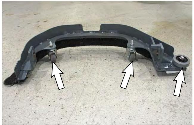
7. Install the caster wheels and the bumper wheel removed from the removed support bracket assembly onto the new support bracket assembly.
