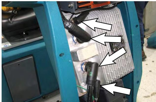
6. Remove the Brain controller from the steering column.
