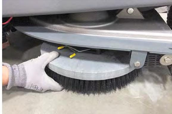
9. Close the side squeegee and the retainer pivot, then insert the pin.
