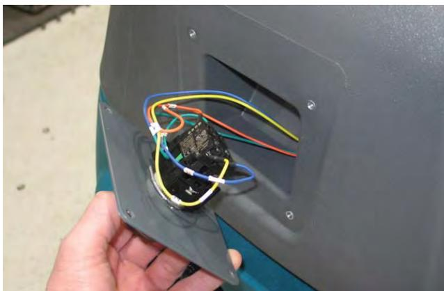
5. Disconnect the harness connections from the blue start/pause button assembly.
