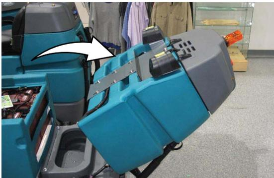
12. Flush the solution tank and rinse the float sensor located inside the back part of the solution tank. Rinse the screen filter on the bottom of the tank.
