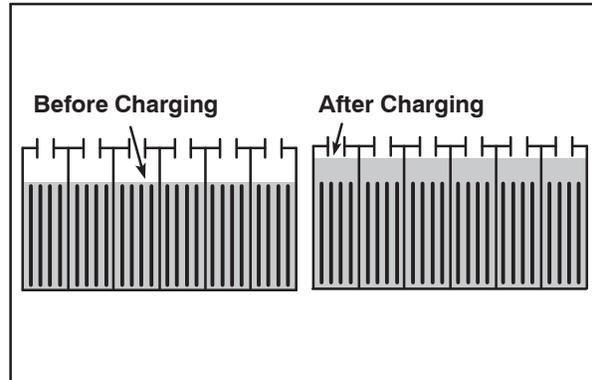
**NOTE: Make sure the battery caps are in place while charging. There may be a sulfur smell after charging batteries. This is normal.**
