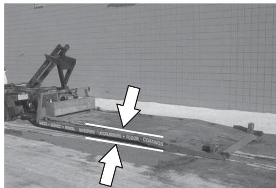
**FOR SAFETY:** When loading machine onto truck or trailer, use winch. Do not drive the machine onto the truck or trailer unless the loading surface is horizontal AND is 380 mm (15 in) or less from the ground.
