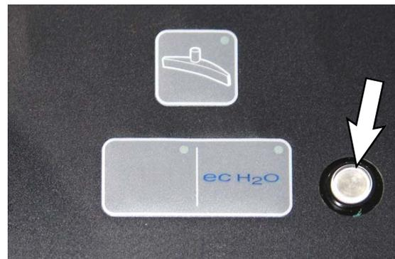
*\*Verify if cleaning detergent was added to solution tank. If ec-H2O system was operated with cleaning detergent, drain solution tank, add clear water and operate the ec-H2O system until the indicator light code clears.*
