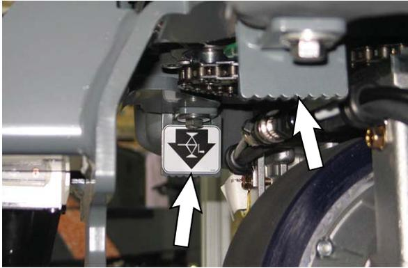
A third location at the front of the machine is located on the back of the LIDAR bracket. **Do Not** position the jack or jack stand at the front of the LIDAR bracket.
