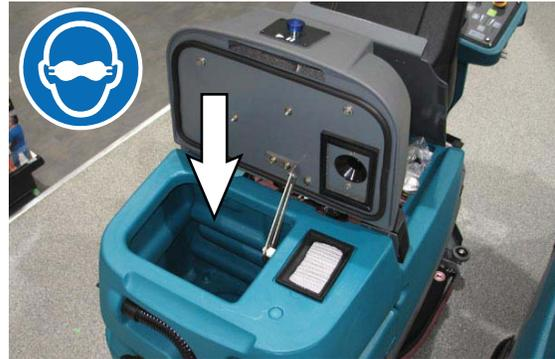
6. Rinse the float sensor located inside the recovery tank.
