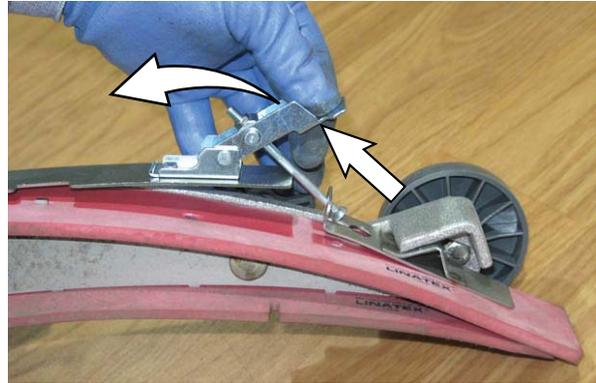
13. Reinstall the rear squeegee under the squeegee mount bracket and tighten all four knobs.
