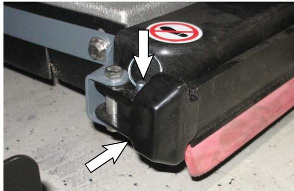
10. If the scrub brush located on the left side of the machine was changed/removed: Close and resecure the left perimeter guard.
