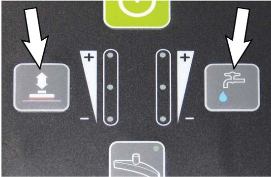
3. Press the *1-Step* button. The light in the button is illuminated. All the preset scrubbing functions will turn on.
