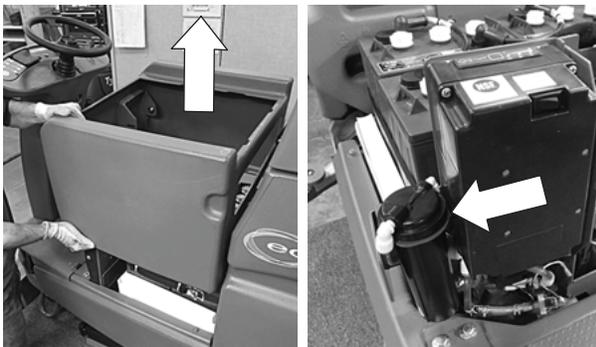
3. Disconnect the two hose connectors from cartridge by pressing the gray collars inward and pulling the connectors outward. Lift cartridge to remove.
