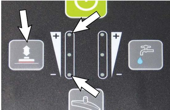
**NOTE:** The machine will operate for a longer time if the *Brush Pressure* and *Solution Flow* settings are set to lowest setting (bottom lights).
