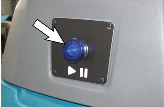
When a saved navigation route is selected on the *UI touchscreen*, press the flashing *blue start/pause button* to begin running the route in robotic mode. If necessary, approach the machine from behind and press the *blue start/pause button* again to pause the in-process robotic route. The machine stops moving forward and the scrub brush stops rotating. The vacuum remains on for a short time to pick up remaining solution and then turns off.
