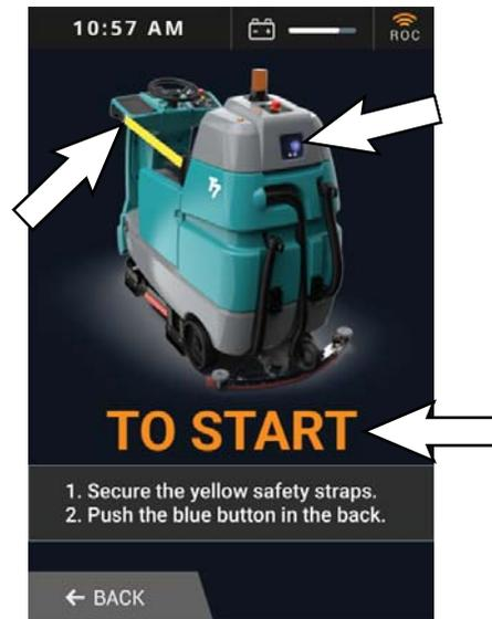
9. Pull the yellow safety straps to the front screws on both sides of the machine.
