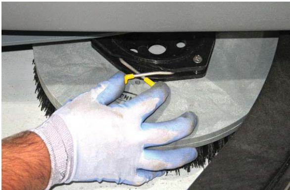
7. Set the yellow spring clip to the open position to make brush installation easier. Press spring clip together and downward to set.
