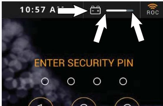
When the batteries are fully charged, the *battery discharge bar* is completely filled. As the batteries discharge, the *battery discharge bar* moves from the right to the left.
