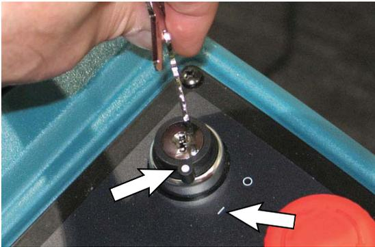
**FOR SAFETY:** While machine is operating in robotic mode, remove key from ON/OFF key switch to prevent unauthorized use without disrupting robotic route.
