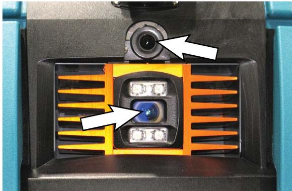
Side 2D and 3D cameras are located on each side of the machine.
