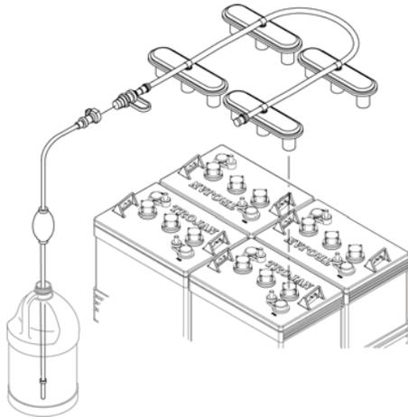
The optional HydroLink battery watering system provides a safe and easy way to maintain the proper electrolyte levels in the batteries. It is designed exclusively for Trojan flooded (wet) lead-acid batteries.
