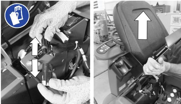
2. Remove the battery compartment shroud from machine to access cartridge.
