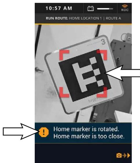
*NOTE: A flashlight can be used in dark and low light areas to help the machine see and scan the home location code.*
