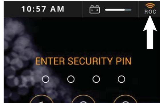
The *ROC indicator* is located on the *UI touchscreen* status bar. When the indicator is orange, the machine is successfully connected to the ROC. If the indicator is gray, the ROC is not connected and cannot be paired with a cell phone.
