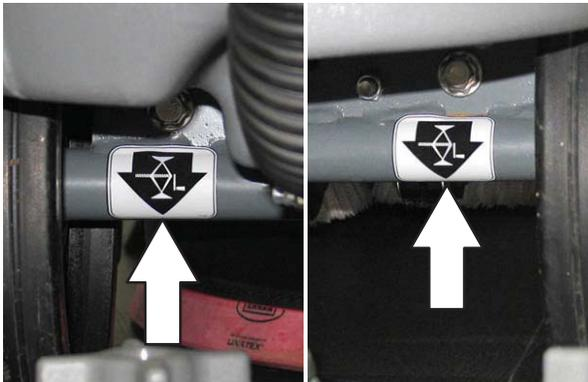
**FOR SAFETY: When servicing machine, block machine tires before jacking machine up. Use a hoist or jack that will support the weight of the machine. Jack machine up at designated locations only. Block machine up with jack stands.**
