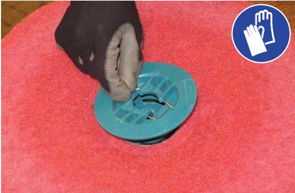
3. Flip or replace the scrub pad, center the scrub pad on the pad driver. Then reinstall the center disk to secure the pad in place on the pad driver.
