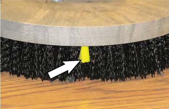
Cleaning pads must be placed on pad drivers before they are ready to use. The cleaning pad is held in place by a pad holder.
