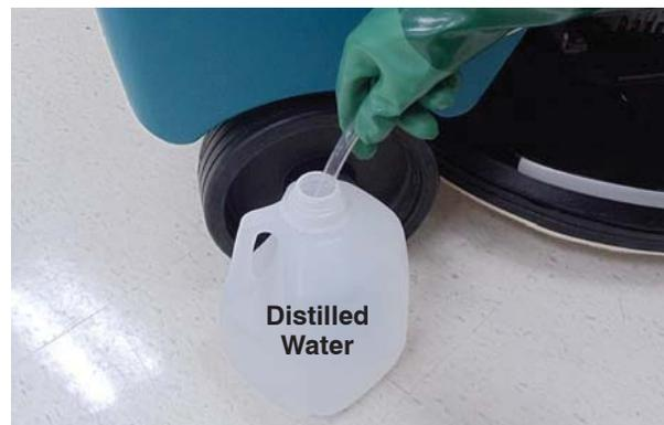
5. Squeeze the bulb on the hand pump hose until firm. The level indicators will turn black when full.
