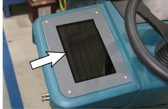
When the machine is turned on, the BrainOS software will automatically initialize. Once initialized, a security pin must be entered to access BrainOS software and use its robotic functionality.
