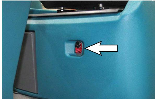
5. The charger will automatically begin charging and shut off when fully charged. The maximum charging cycle may take up to 6-12 hours depending on battery type.
