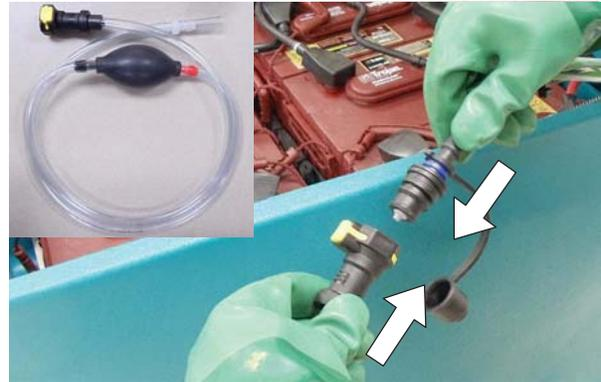
4. Submerge the other end of the hand pump hose into a bottle of distilled water.
