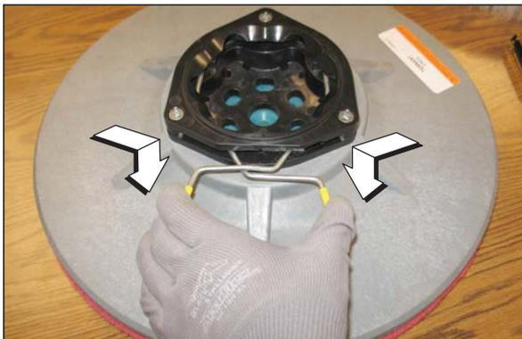
8. Align the pad driver or brush under the motor hub and push it upward to engage hub. Ensure that it is securely mounted onto the motor hub.
