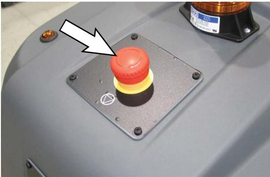
If the *Emergency Stop button* is pressed when the machine is running a robotic route, the in-process route is terminated. Restart the machine by turning the engaged *Emergency Stop button* to the right, and then turning the *ON/OFF key switch* off and back on. Drive the machine to the desired home location code to be scanned, select the desired route, and press the *blue start/pause button* to begin the robotic route.
