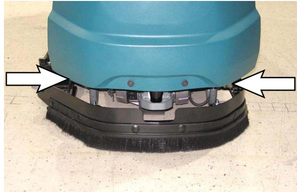
Two front jacking locations are located on the sides of the machine.
