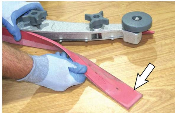
7. Loosen the two outer knobs on the rear squeegee assembly. Remove the front squeegee blade from the squeegee assembly.
