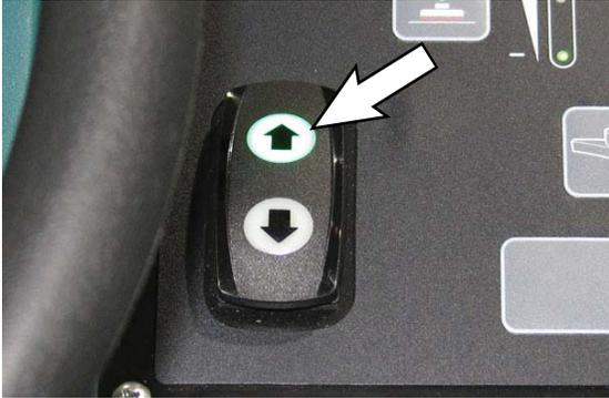
Press the bottom of the *directional switch* to move the machine in reverse. The reverse arrow light located at the bottom of the switch will illuminate when machine placed in the reverse direction.
