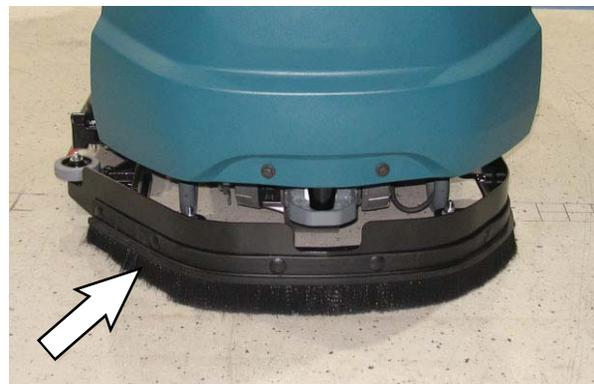
The bristles should lightly touch the floor. Replace damaged and/or worn bristle assemblies.
