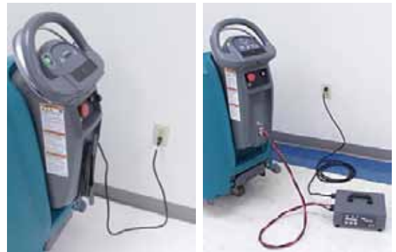
ON- BOARD CHARGER
